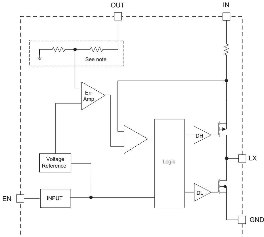
Note: For adjustable version, the internal feedback divider is omitted and the OUT pin is tied directly to the internal error amplifier.
