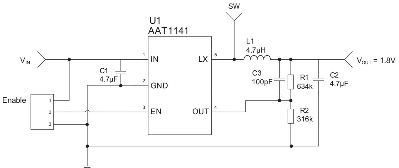
Figure 5: AAT1141 Adjustable Evaluation Board Schematic.
