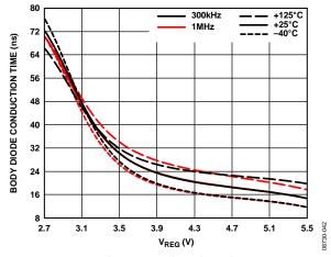
Figure 43. Lower-Side MOSFET Body Diode Conduction Time vs. V<sub>REG</sub>
