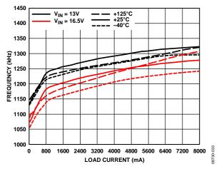
Figure 34. Frequency vs. Load Current, 1.0 MHz,  $V_{OUT} = 5 V$
