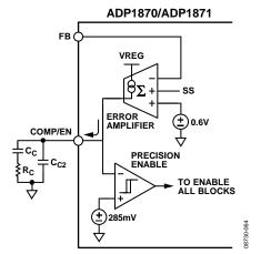
Figure 66. Release COMP/EN Pin to Enable the ADP1870/ADP1871
