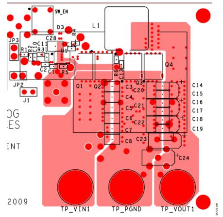
Figure 86. Layer 2 of Evaluation Board
