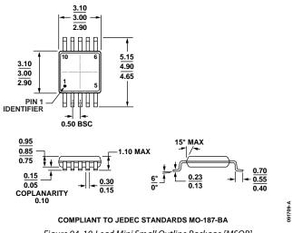
Figure 94. 10-Lead Mini Small Outline Package [MSOP] (RM-10) Dimensions shown in millimeters
