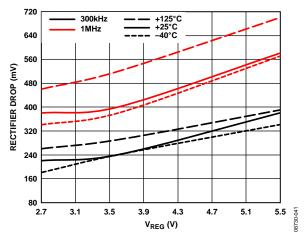
Figure 42. Internal Boost Rectifier Drop vs. V<sub>REG</sub>
