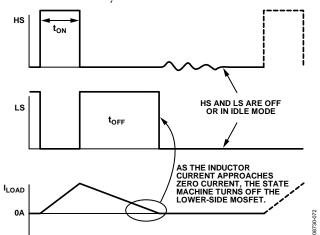
Figure 74. Discontinuous Mode of Operation (DCM)
