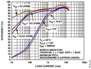
Figure 5. Efficiency—300 kHz,  $V_{OUT} = 1.8 \text{ V}$
