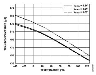
Figure 62. Transconductance (G<sub>m</sub>) vs. Temperature
