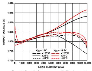
Figure 20. Output Voltage Accuracy—1.0 MHz,  $V_{OUT} = 1.8 \text{ V}$
