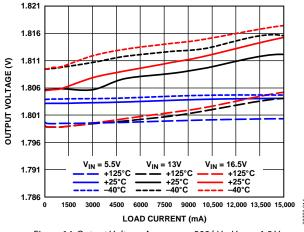
Figure 14. Output Voltage Accuracy—300 kHz,  $V_{OUT} = 1.8 \text{ V}$
