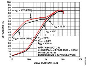
Figure 4. Efficiency—300 kHz,  $V_{OUT} = 0.8 V$
