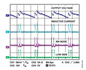
Figure 45. PSM Waveform at Light Load, 500 mA
