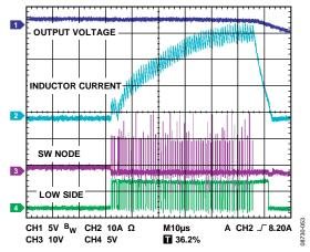
Figure 54. Magnified Waveform During Hiccup Mode
