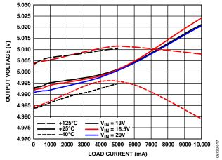
Figure 18. Output Voltage Accuracy—600 kHz,  $V_{OUT} = 5 V$
