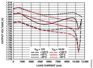
Figure 17. Output Voltage Accuracy—600 kHz, V<sub>OUT</sub> = 1.8 V
