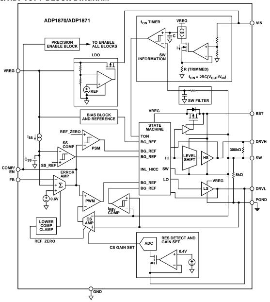
Figure 65. ADP1870/ADP1871 Block Diagram
