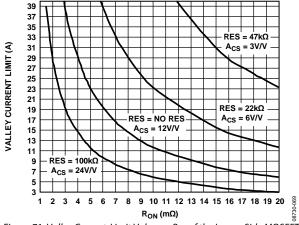
Figure 71. Valley Current-Limit Value vs. R<sub>ON</sub> of the Lower-Side MOSFET for Each Programming Resistor (RES)
