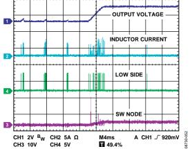
Figure 53. Output Short-Circuit Behavior Leading to Hiccup Mode
