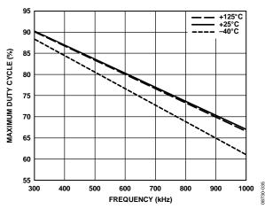
Figure 36. Maximum Duty Cycle vs. Frequency
