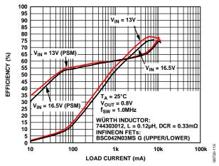
Figure 10. Efficiency—1.0 MHz,  $V_{OUT} = 0.8 \text{ V}$
