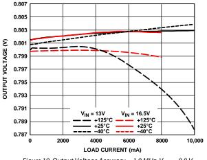
Figure 19. Output Voltage Accuracy—1.0 MHz, V<sub>OUT</sub> = 0.8 V
