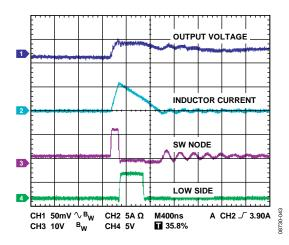
Figure 44. Power Saving Mode (PSM) Operational Waveform, 100 mA
