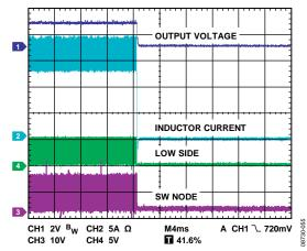
Figure 56. Power-Down Waveform During Heavy Load
