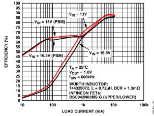
Figure 8. Efficiency—600 kHz,  $V_{OUT} = 1.8 \text{ V}$
