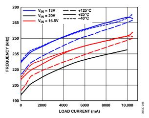
Figure 26. Frequency vs. Load Current, 300 kHz,  $V_{OUT} = 0.8 \text{ V}$
