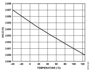
Figure 35. UVLO vs. Temperature
