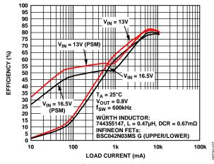
Figure 7. Efficiency—600 kHz,  $V_{OUT} = 0.8 \text{ V}$
