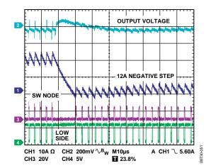
Figure 52. Negative Step During Heavy Load Transient Behavior—Forced PWM at Light Load, 12 A (See Figure 93 Application Circuit)
