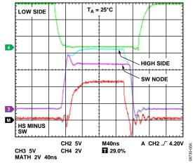
Figure 59. Output Drivers and SW Node Waveforms
