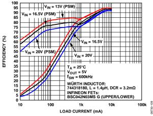
Figure 9. Efficiency—600 kHz,  $V_{OUT} = 5 V$
