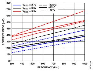
Figure 40. Internal Rectifier Drop vs. Frequency
