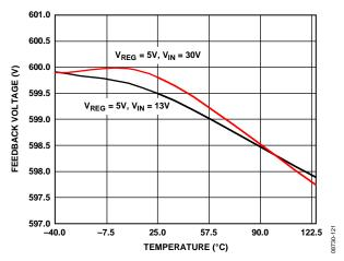
Figure 22. Feedback Voltage vs. Temperature
