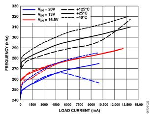
Figure 27. Frequency vs. Load Current, 300 kHz,  $V_{OUT} = 1.8 \text{ V}$
