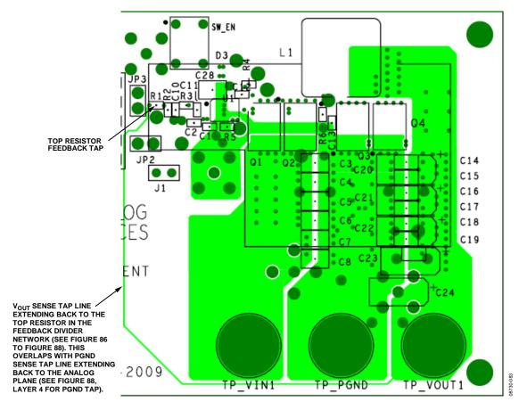
Figure 87. Layer 3 of Evaluation Board
