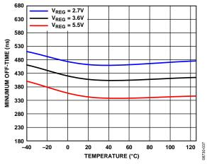
Figure 38. Minimum Off-Time vs. Temperature
