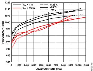
Figure 33. Frequency vs. Load Current, 1.0 MHz,  $V_{OUT} = 1.8 \text{ V}$
