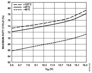
Figure 37. Maximum Duty Cycle vs. High Voltage Input (V<sub>IN</sub>)
