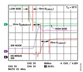
Figure 60. Upper-Side Driver Rising and Lower-Side Falling Edge Waveforms  $(C_{IN} = 4.3 \text{ nF (Upper-/Lower-Side MOSFET)}, Q_{TOTAL} = 27 \text{ nC } (V_{GS} = 4.4 \text{ V } (Q1), V_{GS} = 5 \text{ V } (Q3))$
