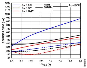
Figure 41. Internal Boost Rectifier Drop vs. V<sub>REG</sub> (Low Input Voltage) Over V<sub>IN</sub> Variation
