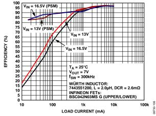
Figure 6. Efficiency—300 kHz, V<sub>OUT</sub> = 7 V
