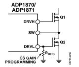
Figure 68. Programming Resistor Location
