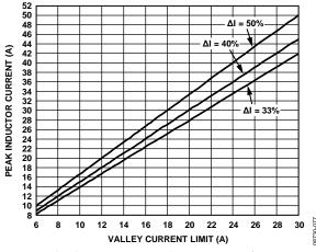
Figure 79. Peak Inductor Current vs. Valley Current Limit for 33%, 40%, and 50% of Inductor Ripple Current
