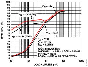
Figure 11. Efficiency—1.0 MHz, V<sub>OUT</sub> = 1.8 V
