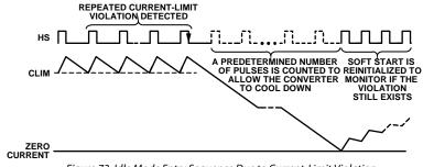
Figure 73. Idle Mode Entry Sequence Due to Current-Limit Violation Rev. 0 | Page 21 of 44
