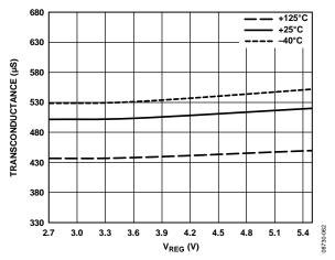
Figure 63. Transconductance (G<sub>m</sub>) vs. V<sub>REG</sub>
