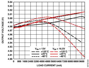
Figure 21. Output Voltage Accuracy—1.0 MHz,  $V_{OUT} = 5 V$
