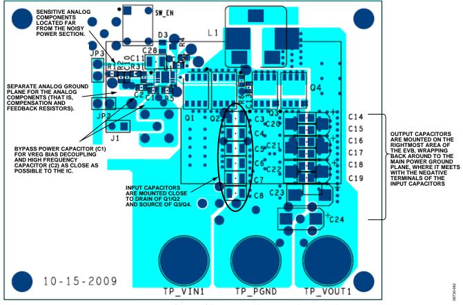
Figure 85. Overall Layout of the ADP1870 High Current Evaluation Board
