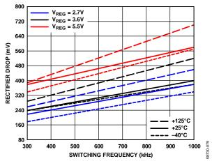
Figure 81. Internal Rectifier Voltage Drop vs. Switching Frequency
