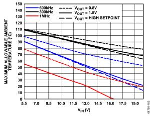
Figure 83. Ambient Temperature vs. V<sub>IN</sub> for 10-Lead MSOP (171°C/W), 4-Layer EVB, CIN = 4.3 nF (Upper-/Lower-Side MOSFET)
