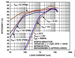
Figure 2. Efficiency vs. Load Current (Vout = 1.8 V, 300 kHz)
