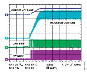
Figure 55. Start-Up Behavior at Heavy Load, 12 A, 300 kHz (See Figure 93 Application Circuit)
