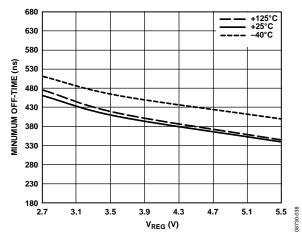
Figure 39. Minimum Off-Time vs. V<sub>REG</sub> (Low Input Voltage)
