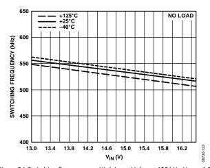
Figure 24. Switching Frequency vs. High Input Voltage, 600 kHz,  $V_{OUT} = 1.8 V$ ,  $V_{IN}$  Range = 13 V to 16.5 V
