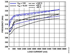
Figure 28. Frequency vs. Load Current, 300 kHz, Vout = 7 V
