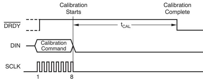
Figure 62. Calibration Command
