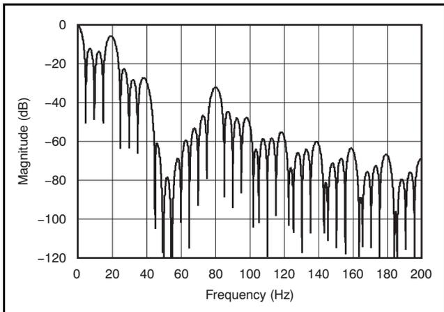
Figure 34. Filter Profile with Data Rate = 5SPS
