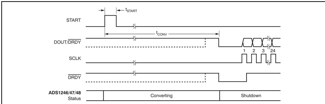
Figure 47. Timing for Single Conversion Using START Pin
