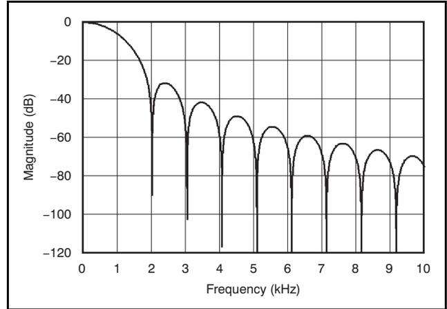
Figure 43. Filter Profile with Data Rate = 1kSPS
