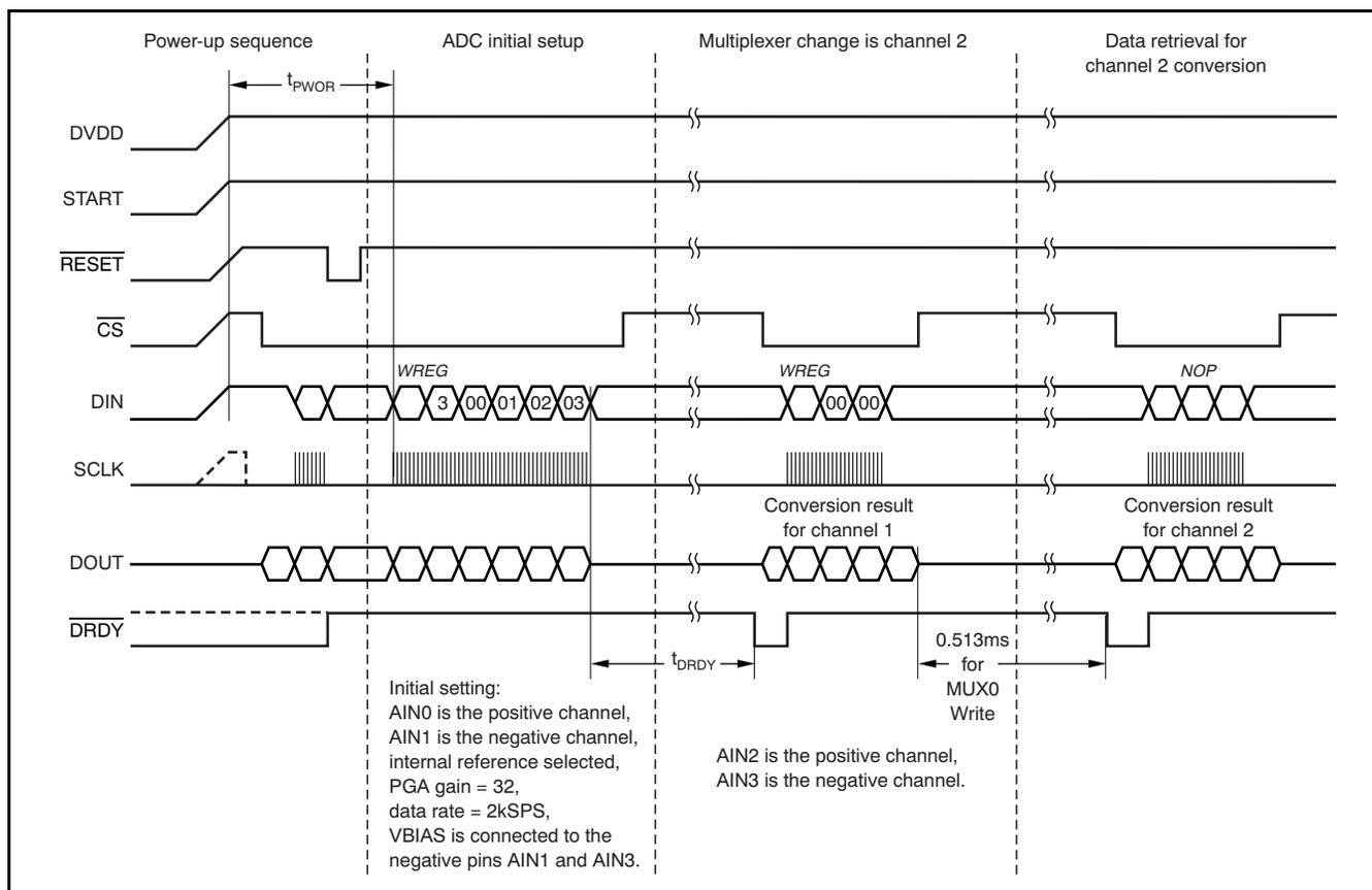
Figure 63. SPI Communication Sequence for Channel Multiplexing
