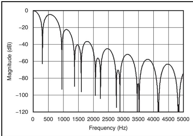
Figure 41. Filter Profile with Data Rate = 320SPS
