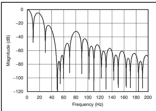
Figure 35. Filter Profile with Data Rate = 10SPS
