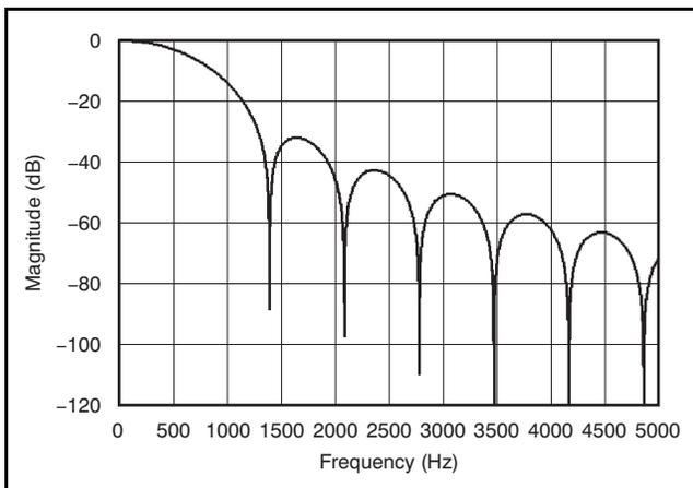
Figure 42. Filter Profile with Data Rate = 640SPS
