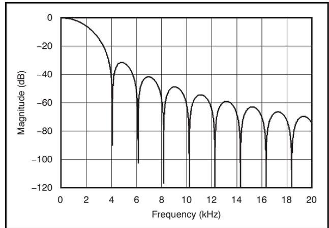
Figure 44. Filter Profile with Data Rate = 2kSPS
