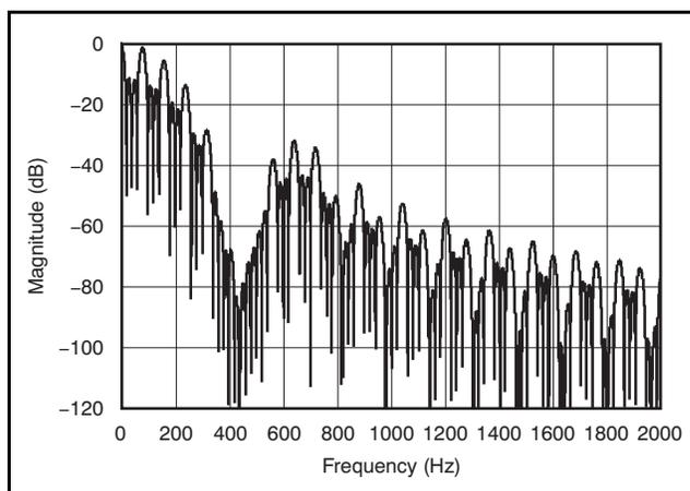
Figure 38. Filter Profile with Data Rate = 40SPS
