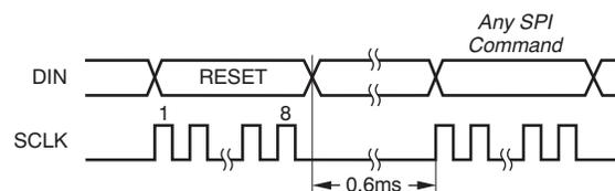
Figure 55. SPI Communication After an SPI Reset
