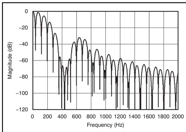
Figure 39. Filter Profile with Data Rate = 80SPS
