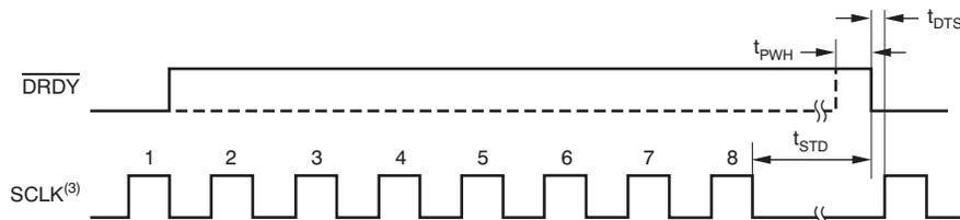
Figure 2. SPI Interface Timing to Allow Conversion Result Loading<sup>(3)(4)</sup>
