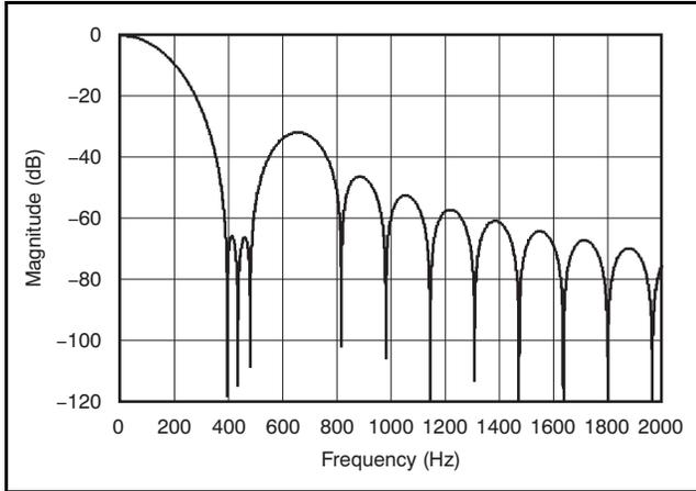
Figure 40. Filter Profile with Data Rate = 160SPS
