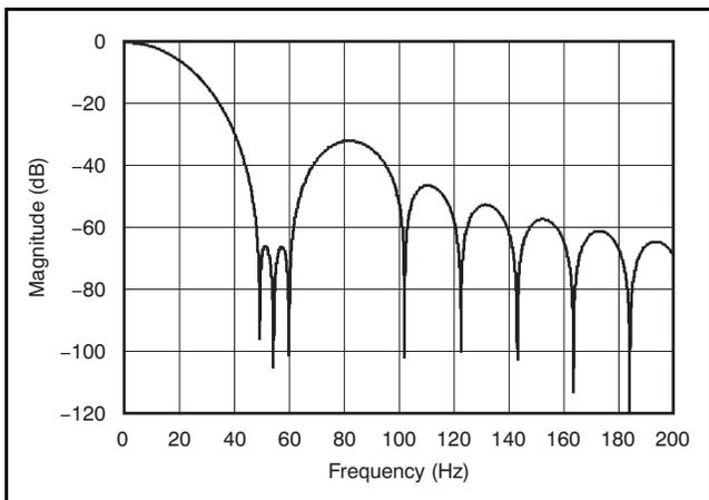
Figure 36. Filter Profile with Data Rate = 20SPS
