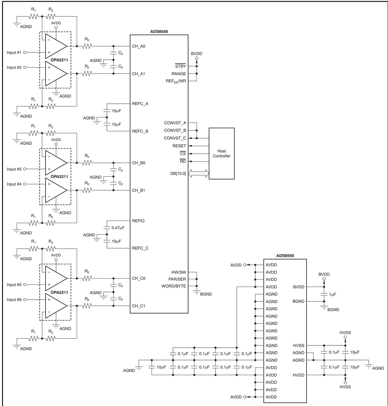
Figure 43. Minimum Configuration in Parallel Interface Mode
