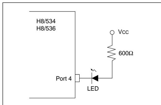
**Figure 20-2 Example of Circuit for Driving an LED**
