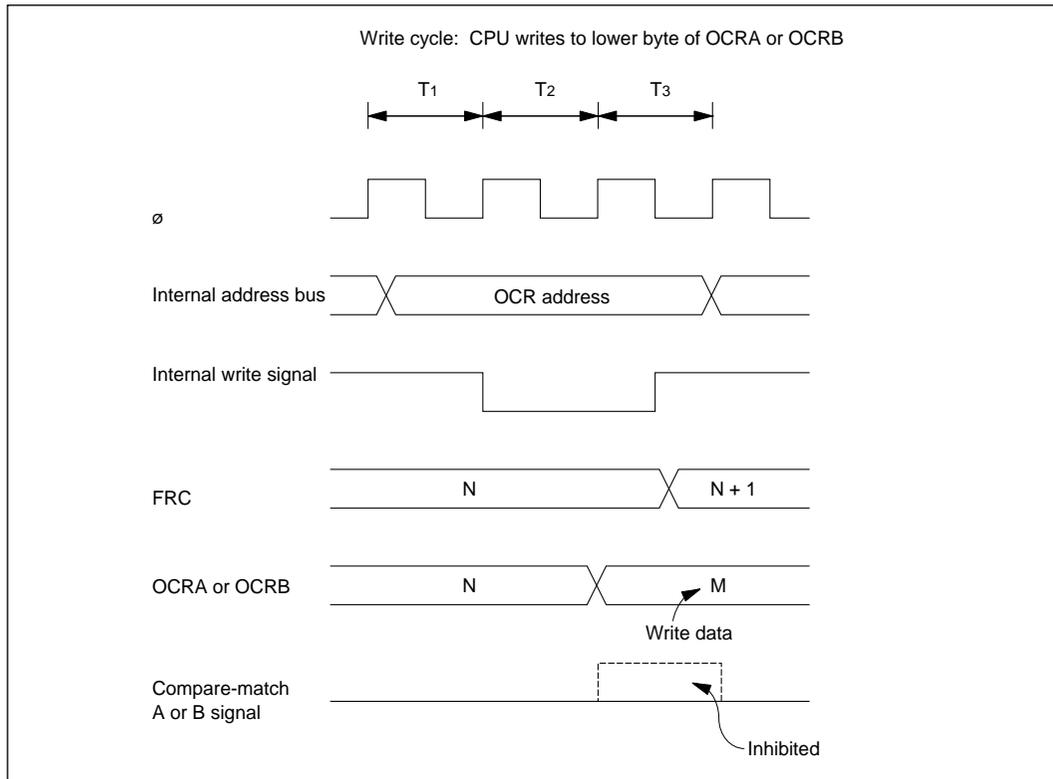
**Figure 10-14 Contention between OCR Write and Compare-Match**
