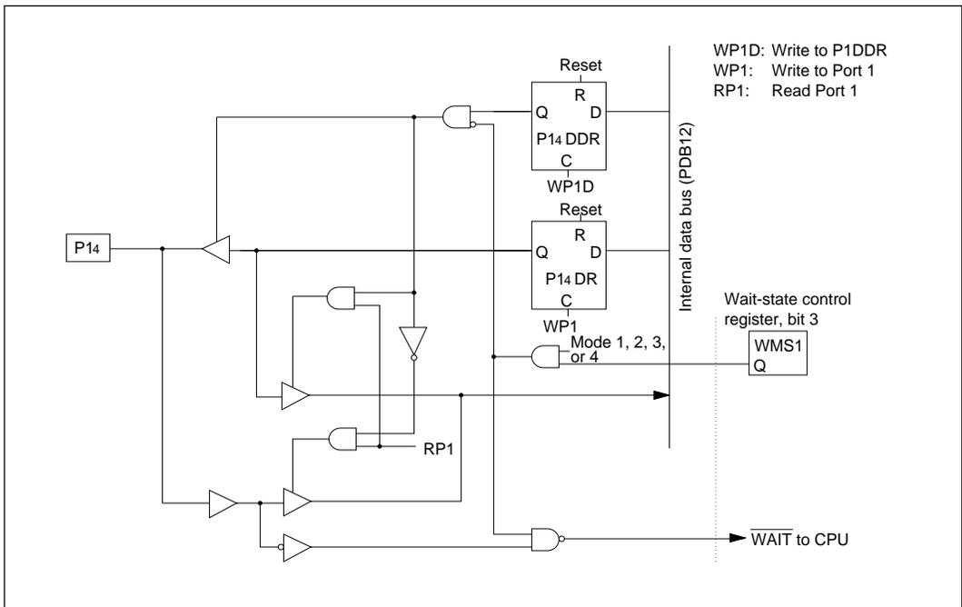
**Figure C-1 (e) Schematic Diagram of Port 1, Pin P14**
