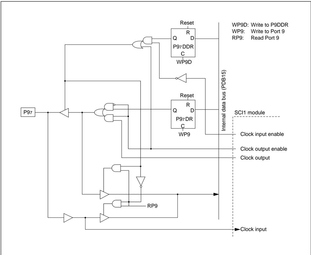
**Figure C-9 (g) Schematic Diagram of Port 9, Pin P97**
