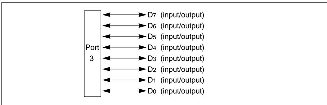
**Figure 9-6 Port 3 Pin Functions in Expanded Modes**
