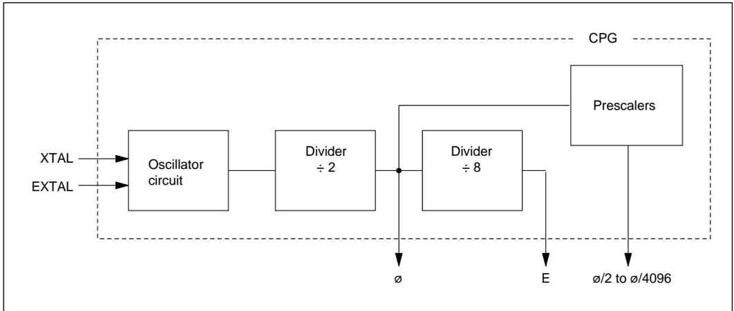
Figure 8-1 Block Diagram of Clock Pulse Generator
