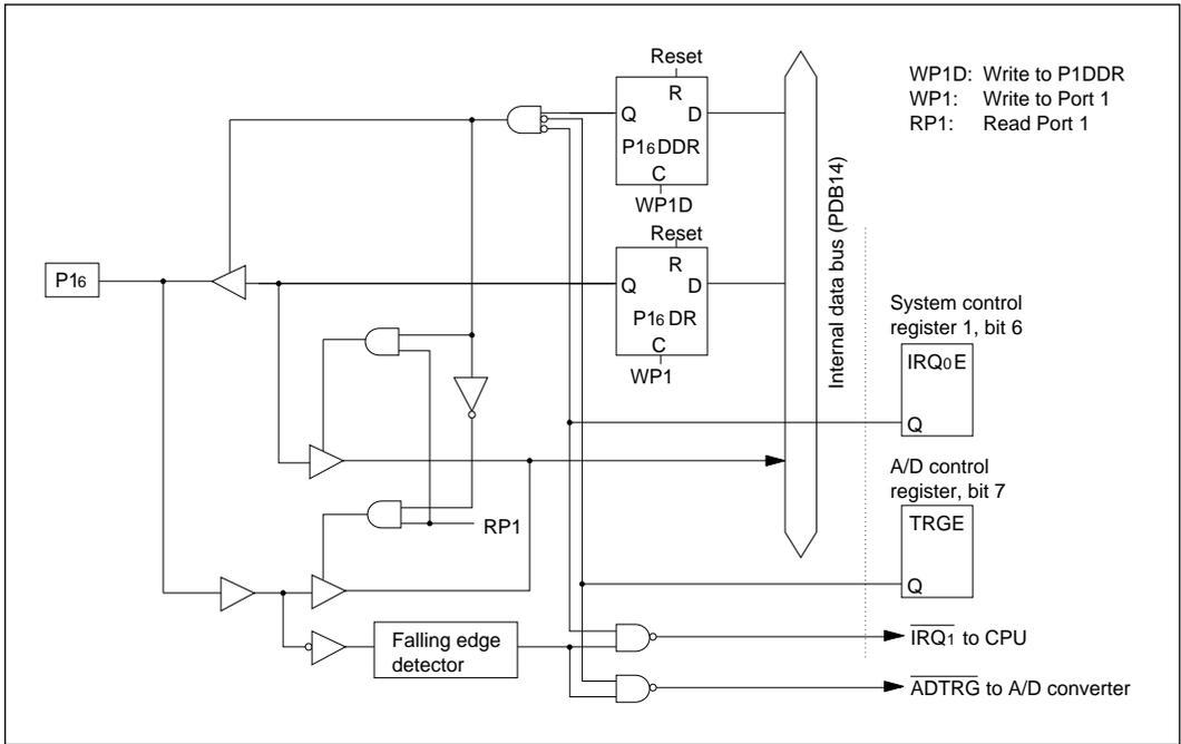
**Figure C-1 (g) Schematic Diagram of Port 1, Pin P16**
