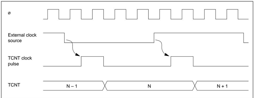
**Figure 11-2 Count Timing for External Clock Input**
