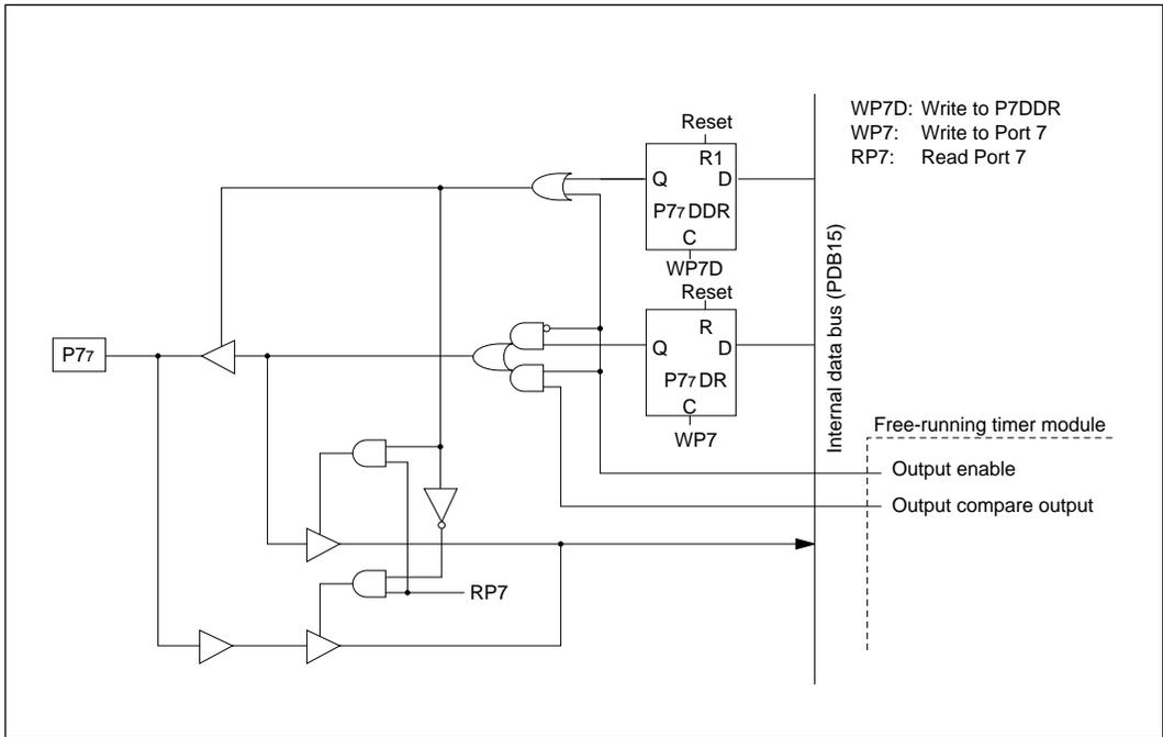
**Figure C-7 (e) Schematic Diagram of Port 7, Pin P77**
