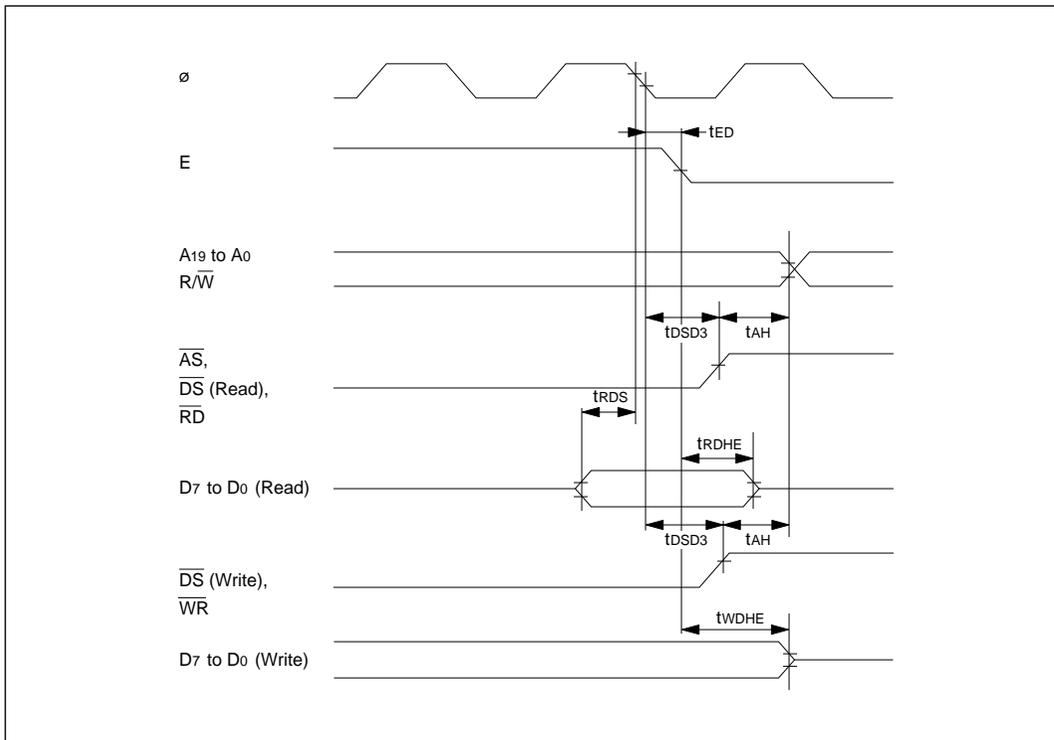
**Figure 20-6 Bus Cycle Synchronized with E Clock**
