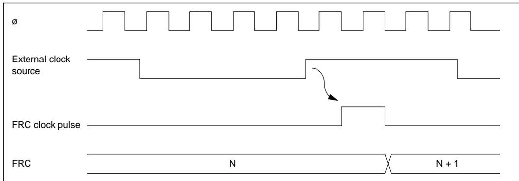
**Figure 10-3 Increment Timing for External Clock Input**
