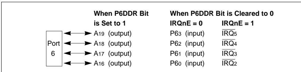
**Figure 9-17 Port 6 Pin Functions in Mode 4**
