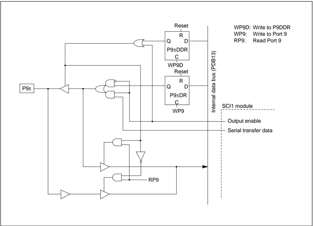
**Figure C-9 (e) Schematic Diagram of Port 9, Pin P95**
