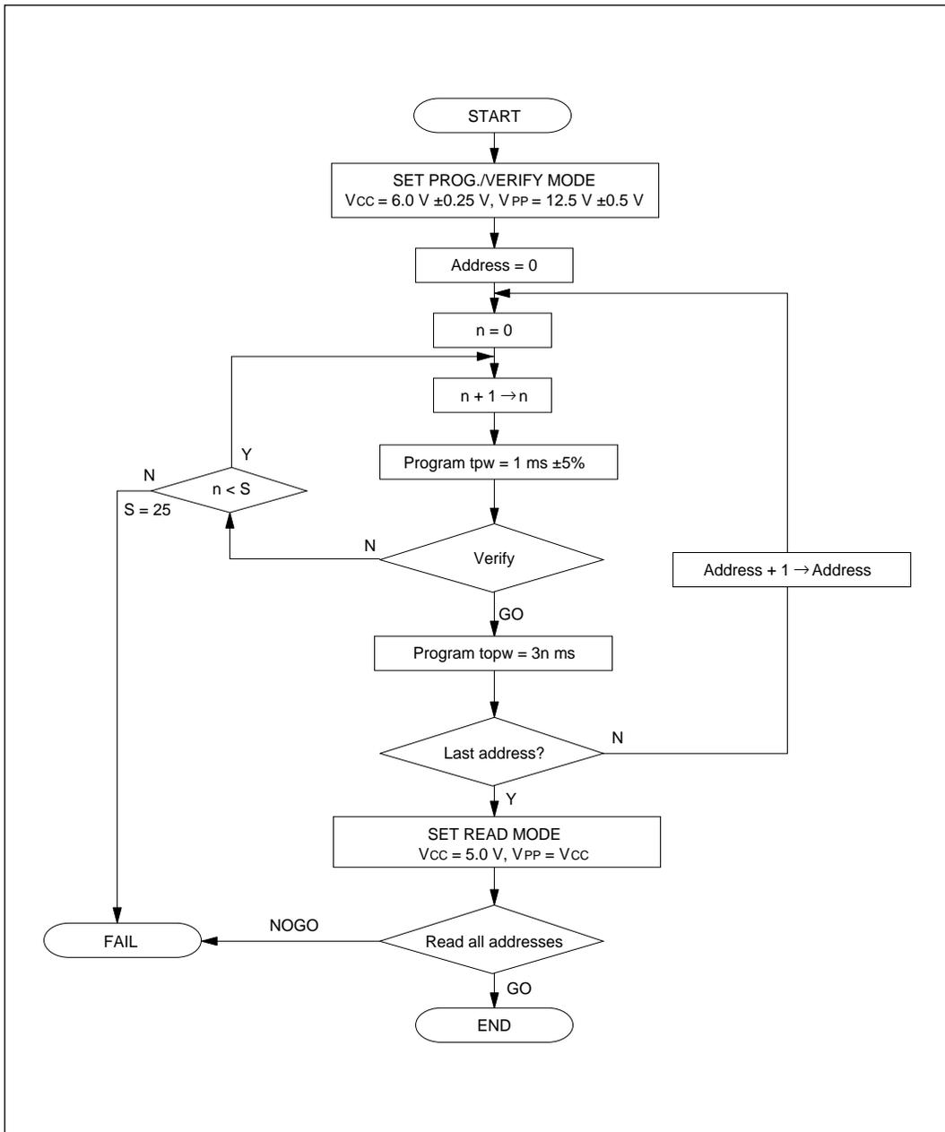
Figure 17-4 High-Speed Programming Flowchart (H8/534)
