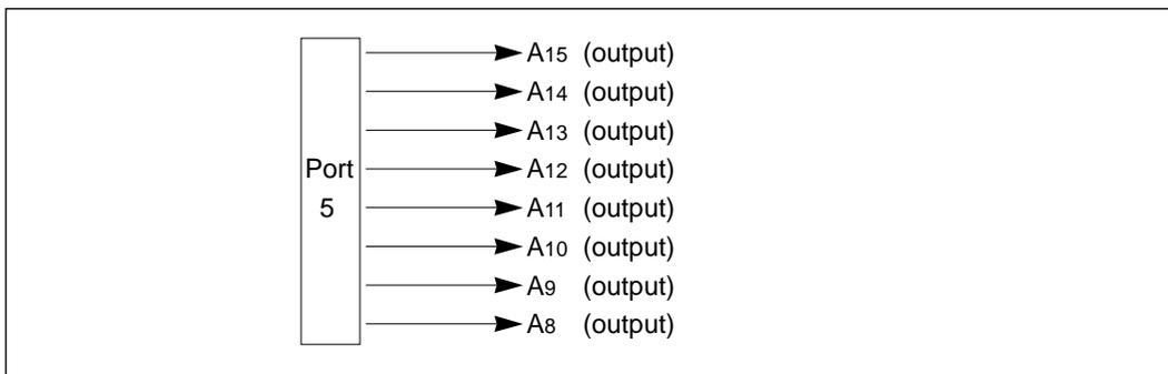
**Figure 9-12 Port 5 Pin Functions in Modes 1 and 3**
