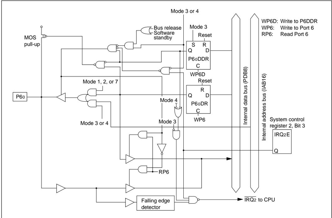
Figure C-6 (a) Schematic Diagram of Port 6, Pin P60
