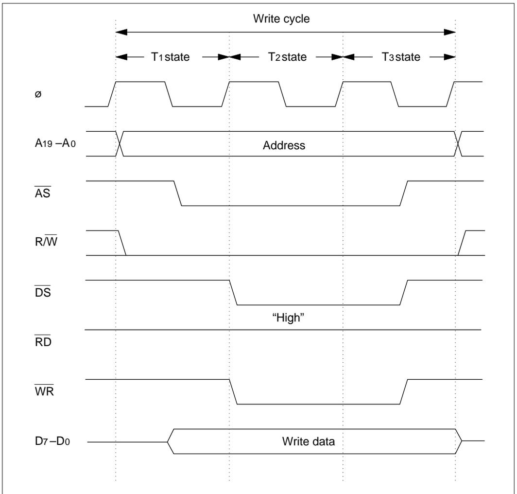
**Figure 3-10 (b) External Access Cycle (Write Access)**
