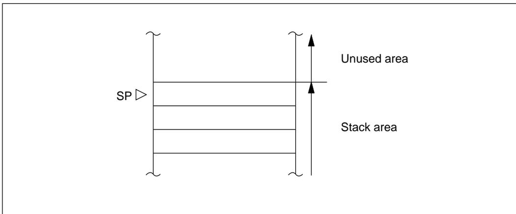
**Figure 3-3 Stack Pointer**
