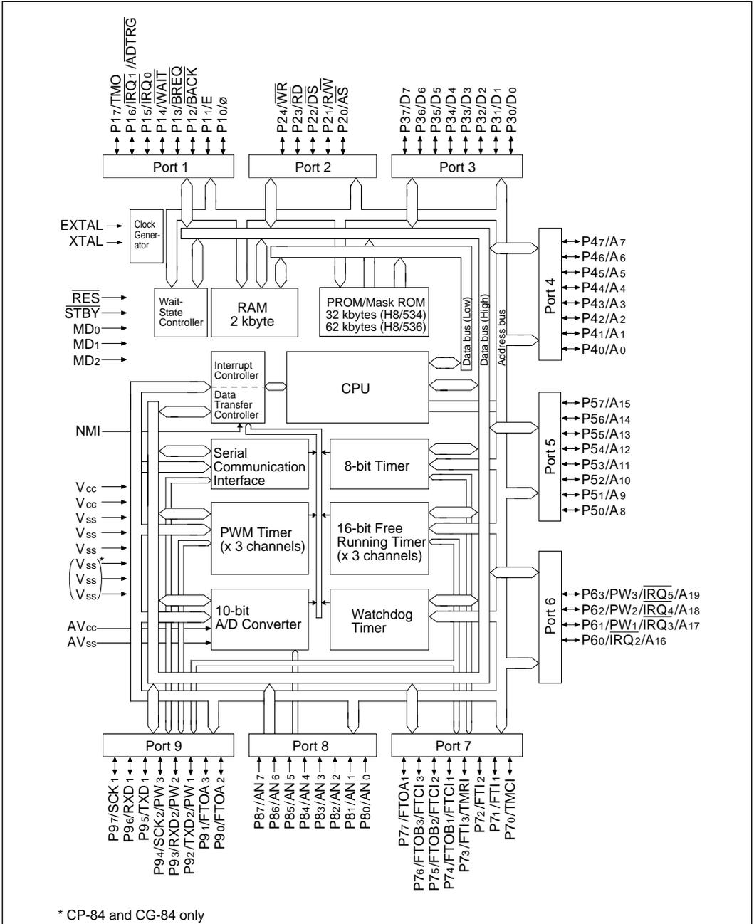
Figure 1-1 Block Diagram
