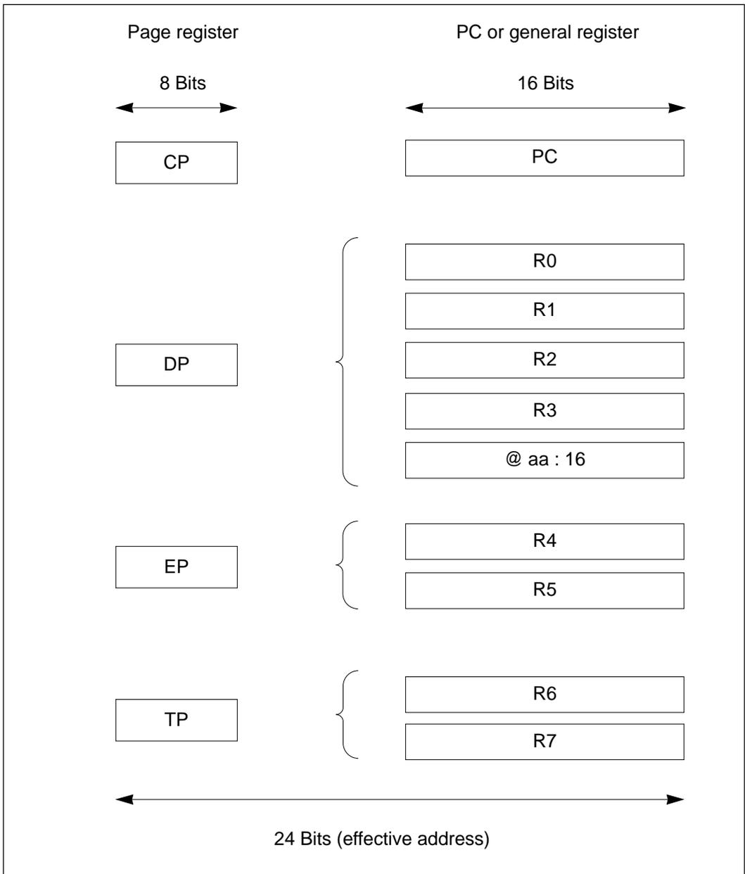
**Figure 3-4 Combinations of Page Registers with Other Registers**
