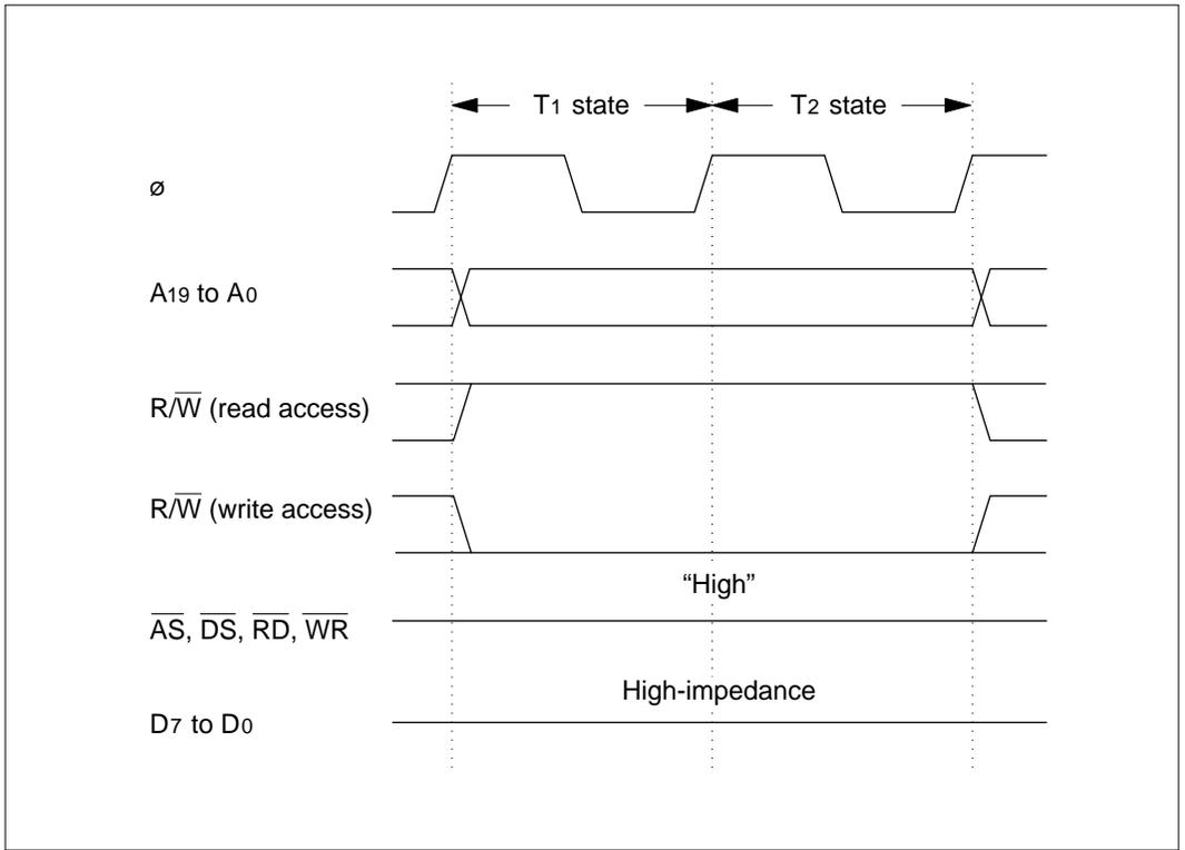
**Figure 3-7 Pin States during Access to On-Chip Memory**
