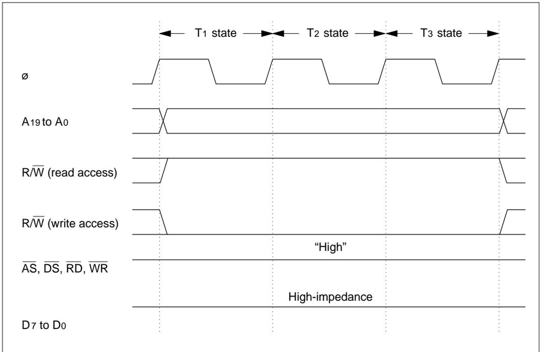
Figure 3-9 Pin States during Register Field Access
