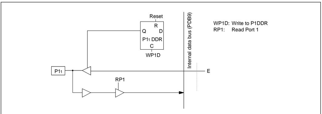
Figure C-1 (b) Schematic Diagram of Port 1, Pin P11
