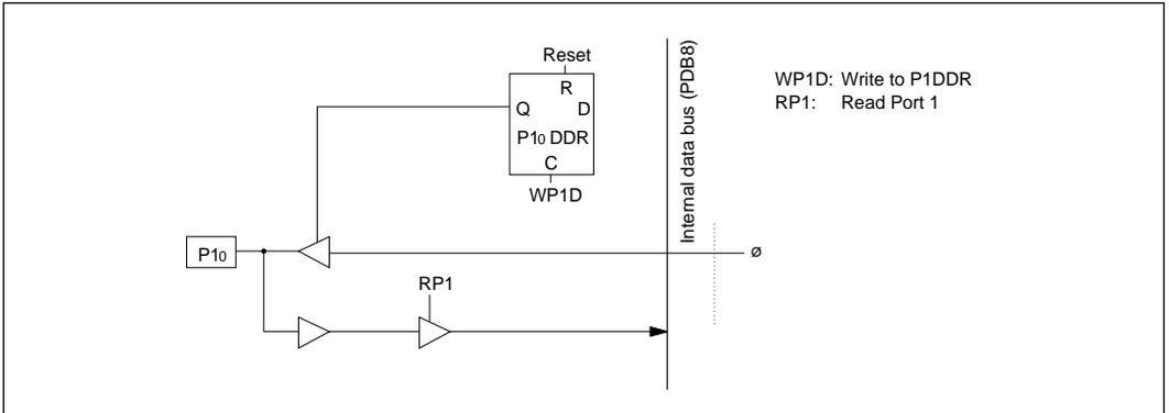
Figure C-1 (a) Schematic Diagram of Port 1, Pin P10
