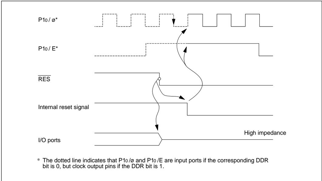
**Figure E-5 Reset during Memory Access (Mode 7)**
