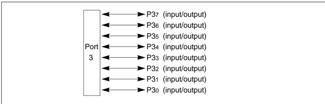
**Figure 9-7 Port 3 Pin Functions in Single-Chip Mode**
