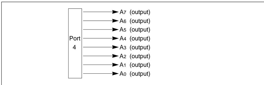
**Figure 9-9 Port 4 Pin Functions in Expanded Modes**
