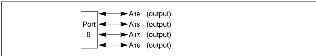
**Figure 9-16 Port 6 Pin Functions in Mode 3**
