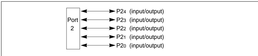
**Figure 9-4 Port 2 Pin Functions in Single-Chip Mode**
