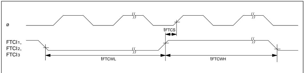
Figure 20-15 External Clock Input Timing for Free-Running Timers
