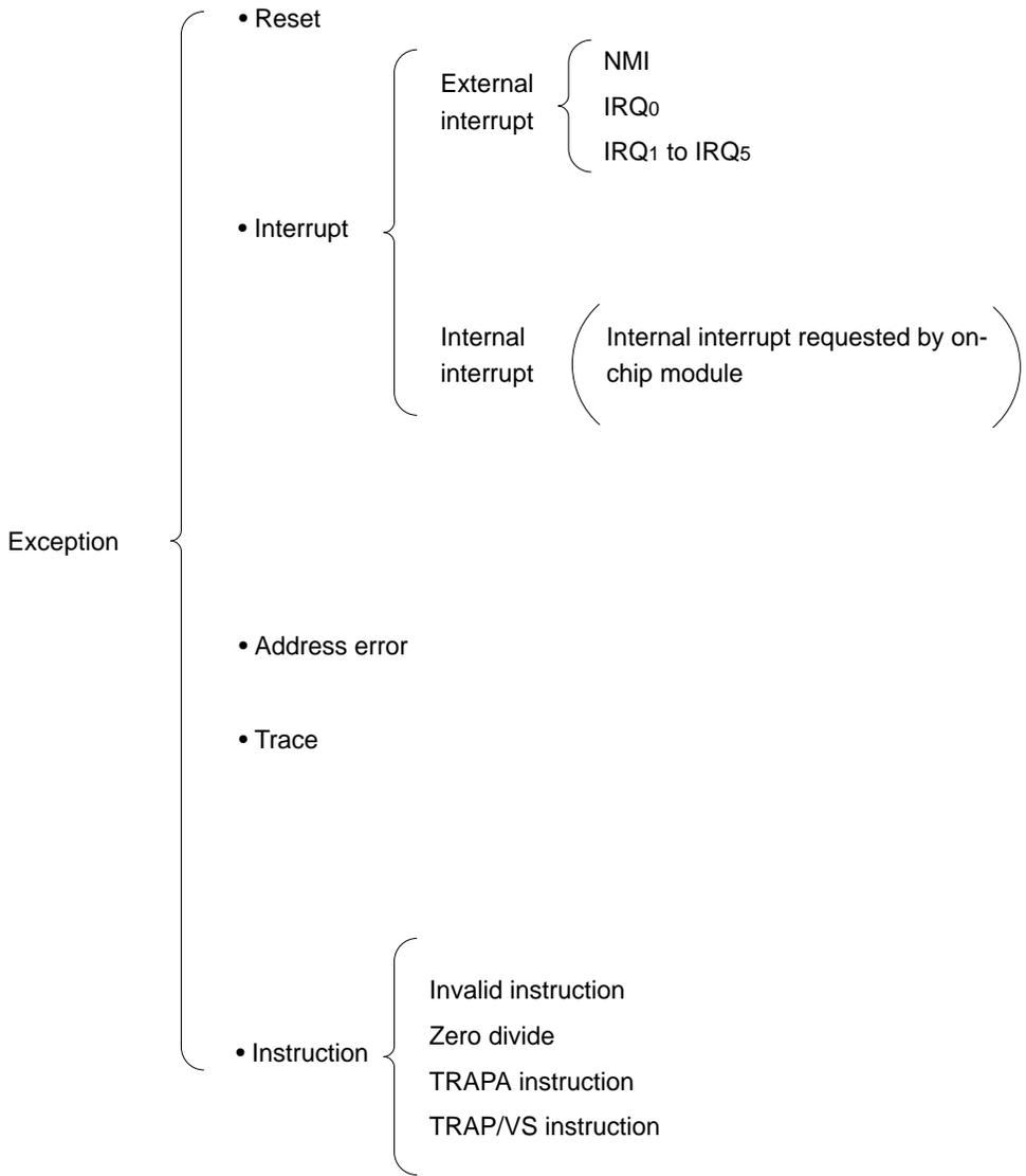
**Figure 4-1 Types of Factors Causing Exception Handling**
