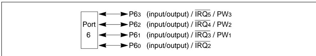
**Figure 9-18 Port 6 Pin Functions in Modes 7, 2, and 1**
