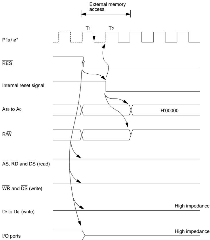
\* The dotted line indicates that P10/ø is an input port if the corresponding DDR bit is 0, but a clock output pin if the DDR bit is 1.
