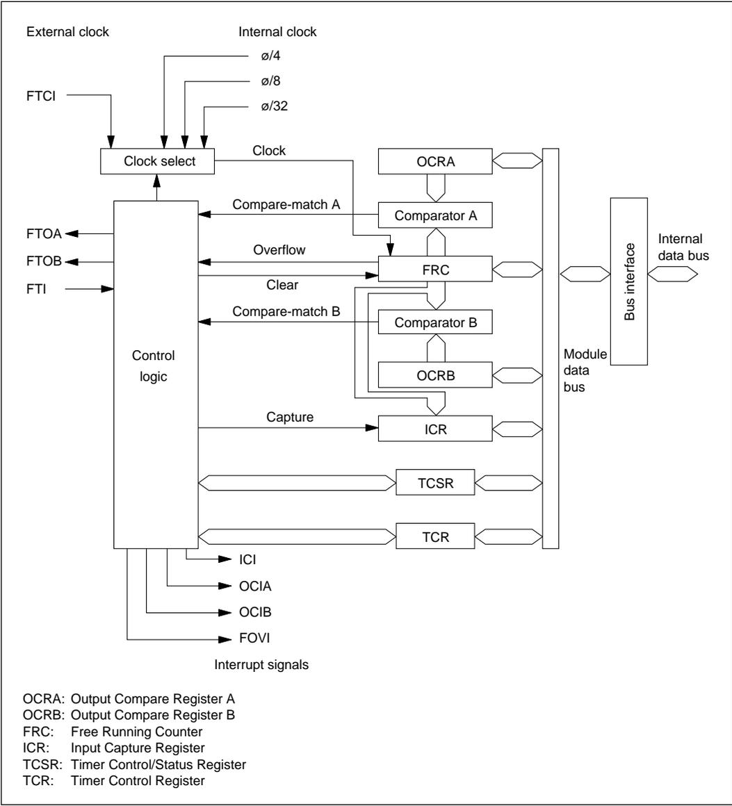
**Figure 10-1 Block Diagram of 16-Bit Free-Running Timer**
