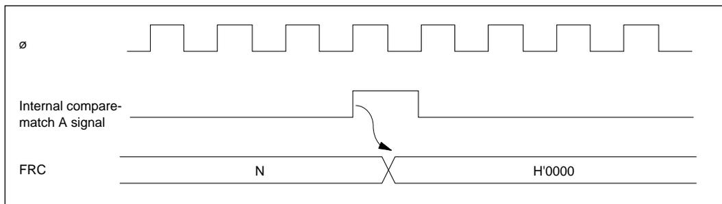
**Figure 10-6 Clearing of FRC by Compare-Match A**
