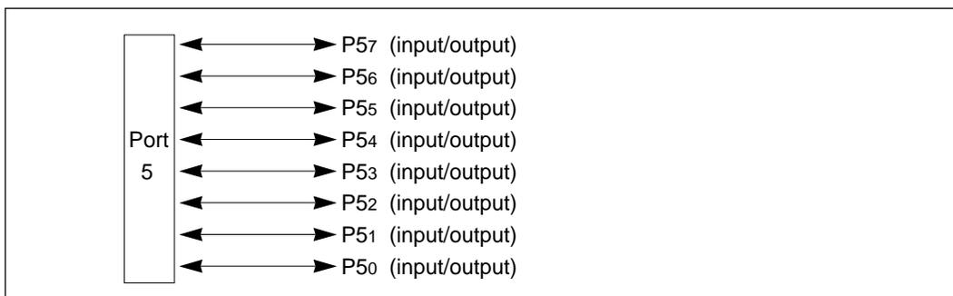
**Figure 9-14 Port 5 Pin Functions in Single-Chip Mode**
