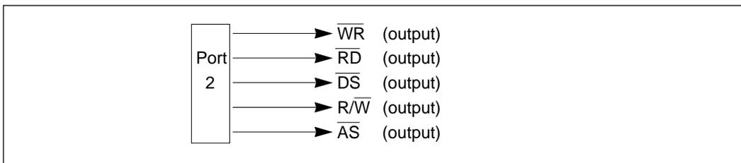
**Figure 9-3 Port 2 Pin Functions in Expanded Modes**
