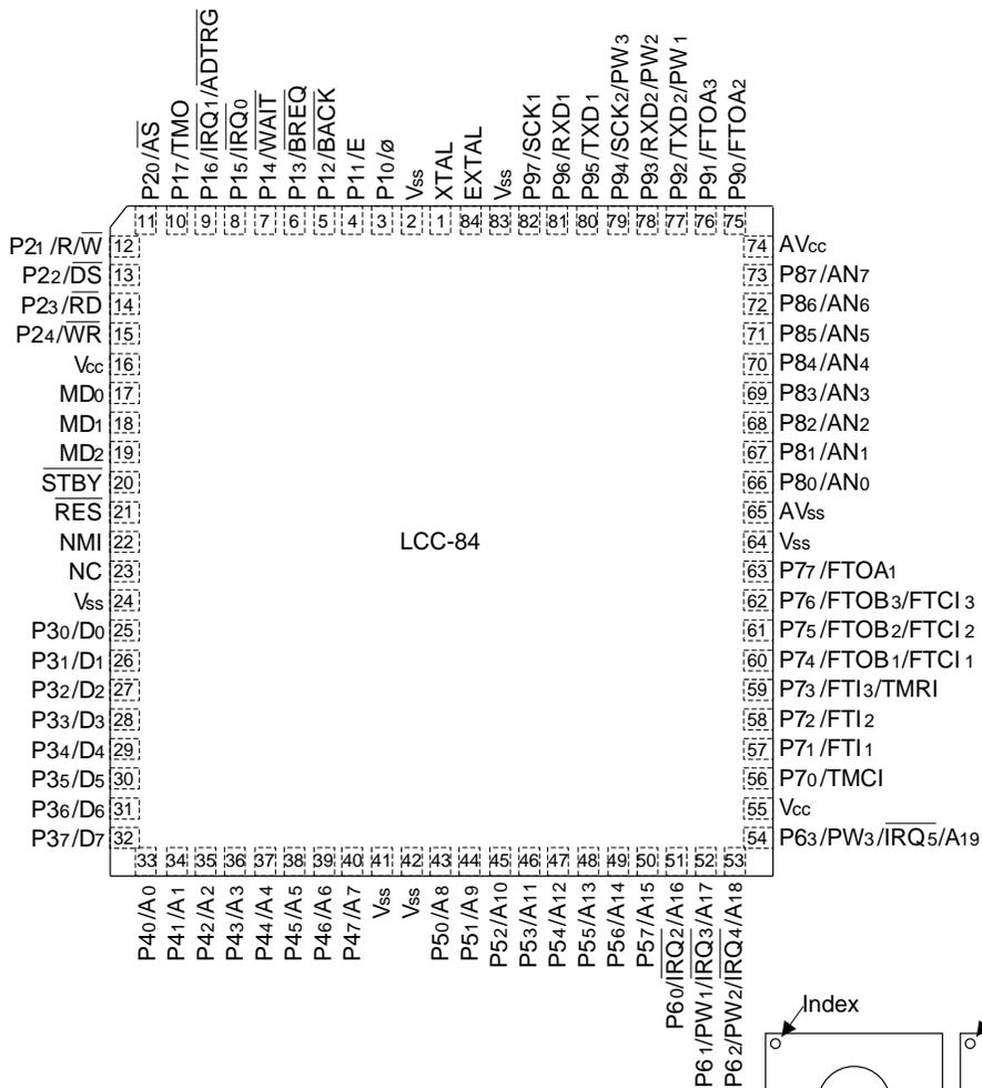
Figure 1-3 Pin Arrangement (CG-84, Top View)
