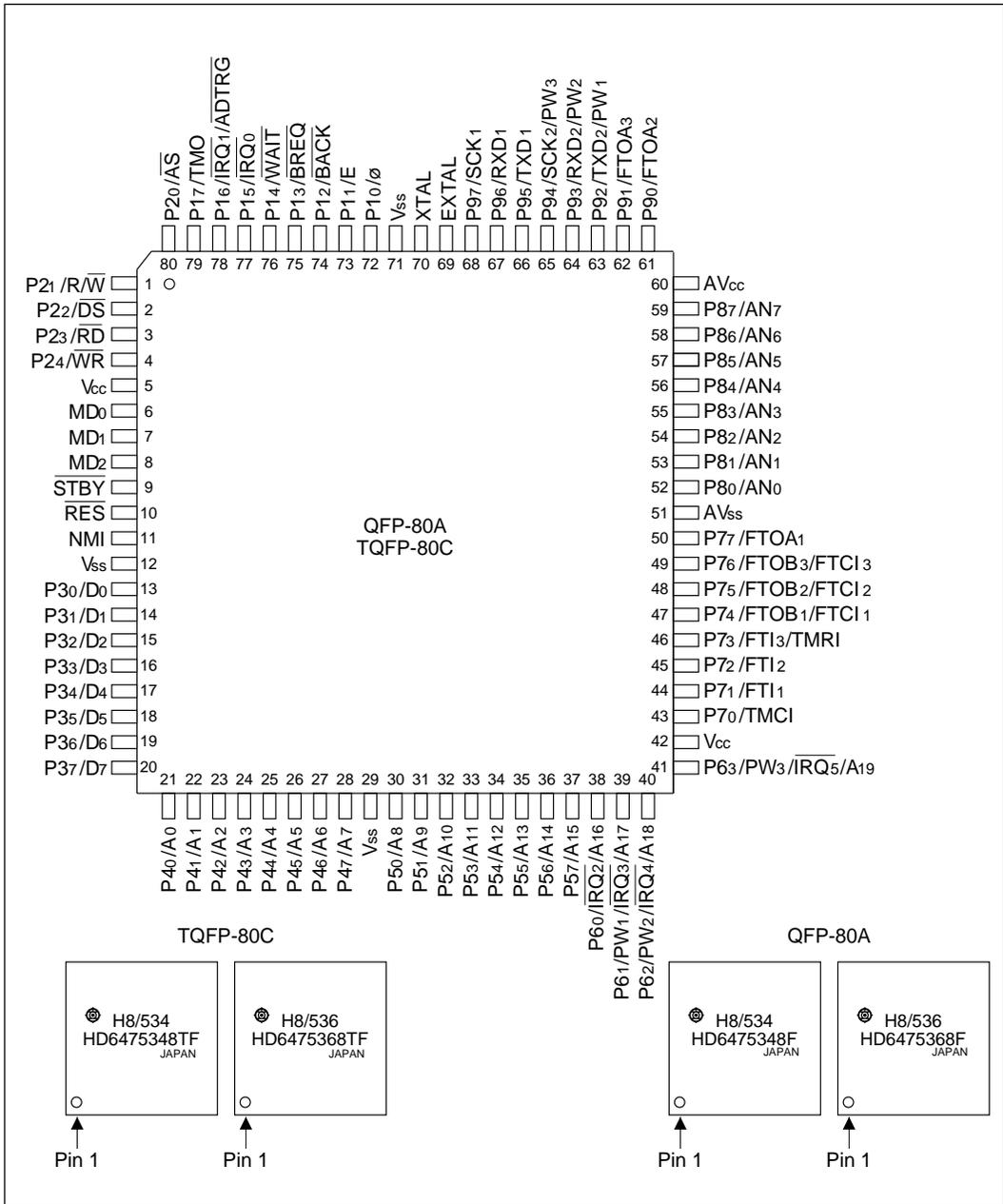
Figure 1-4 Pin Arrangement (FP-80A, TFP-80C, Top View)
