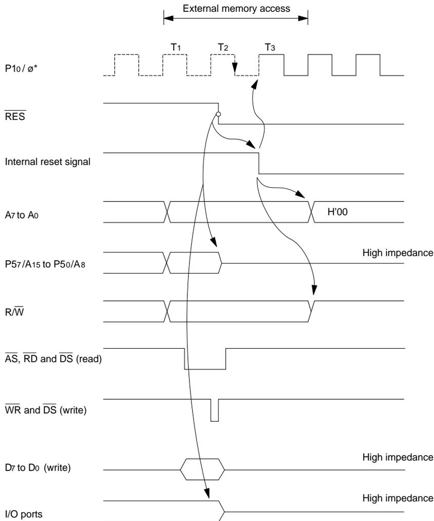
\* The dotted line indicates that P10/ $\phi$  is an input port if the corresponding DDR bit is 0, but a clock output pin if the DDR bit is 1.
