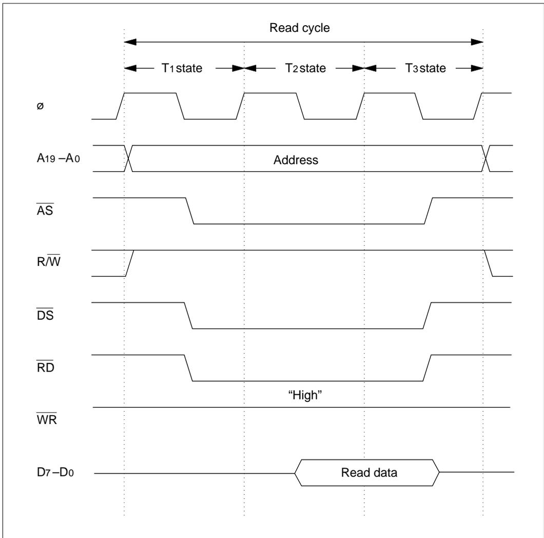
Figure 3-10 (a) External Access Cycle (Read Access)
