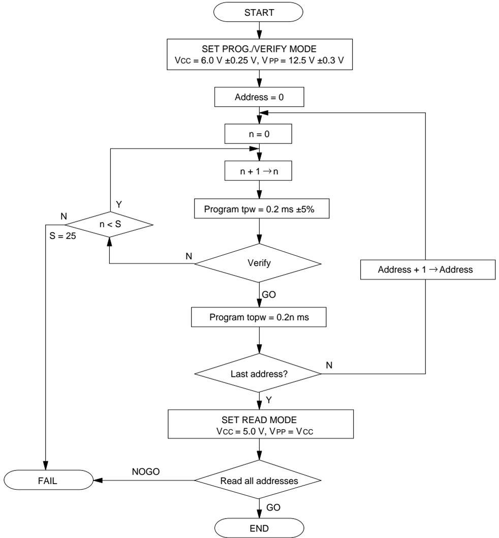
**Figure 17-6 High-Speed Programming Flowchart (H8/536)**
