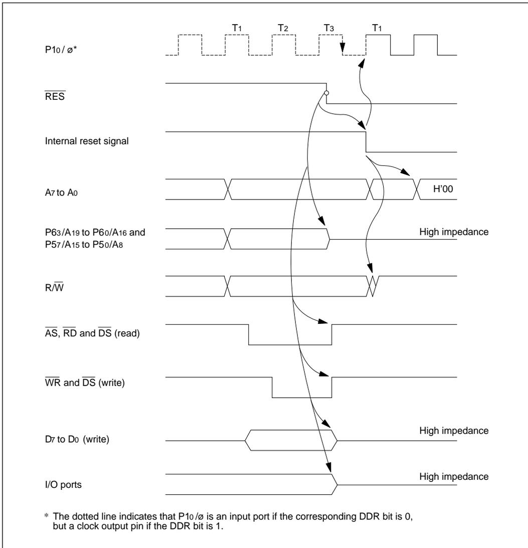
**Figure E-4 Reset during Memory Access (Mode 4)**
