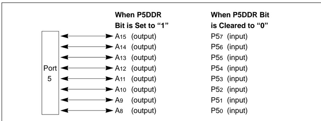
**Figure 9-13 Port 5 Pin Functions in Modes 2 and 4**
