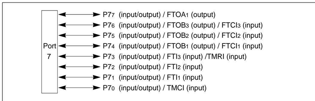
**Figure 9-19 Pin Functions of Port 7**
