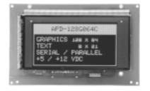
The APD-128G064C is a dot matrix graphic display with an array of  $128 \times 64$  pixels available. The module is composed of a highly reliable DC plasma display, ASCII input graphics controller, DC converter and drive circuitry which are assembled to form a rugged, slim profile display sub-system.
