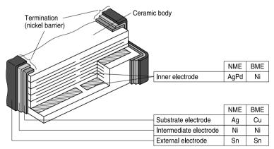
NME: Noble Metal Electrode BME: Base Metal Electrode
