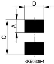
**Recommended dimensions (mm) for reflow soldering**
