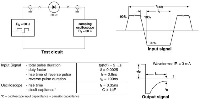
\*C = oscilloscope input capactitance + parasitic capacitance
