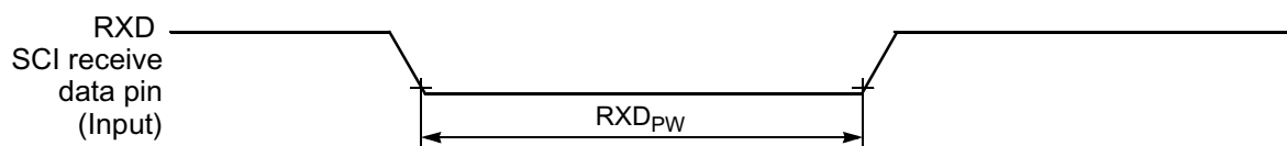
Figure 10-16 RXD Pulse Width
