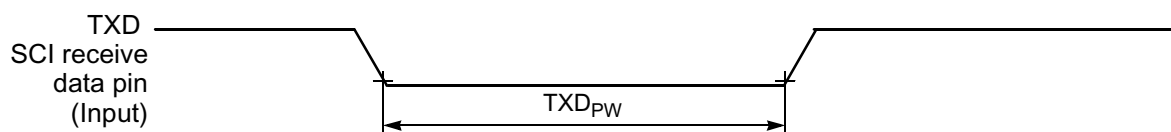
Figure 10-17 TXD Pulse Width
