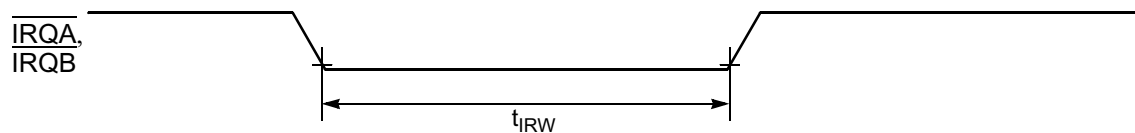
Figure 10-6 External Interrupt Timing (Negative-Edge Sensitive)
