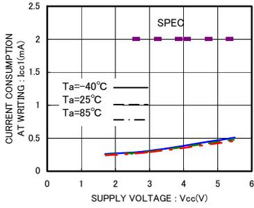
Fig.9 Current consumption at WRITE operation  $I_{cc1}$  (fsc1=400kHz)
