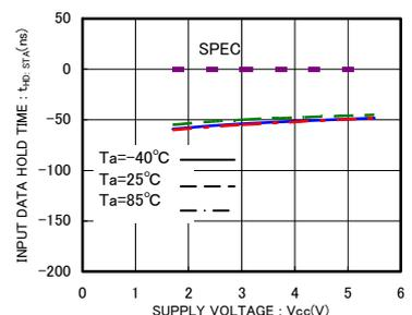
Fig.17 Input Data Hold Time  $t_{HD:DAT(HIGH)}$
