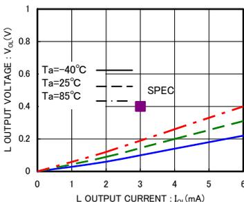
Fig.6 'L' output voltage  $V_{OL}$ - $I_{OL}$  ( $V_{CC}=2.5V$ )
