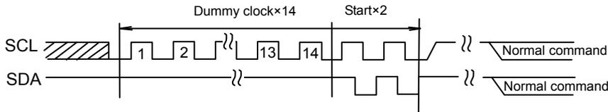
Fig.38-(a) The case of 14 Dummy clock + START + START+ command input
