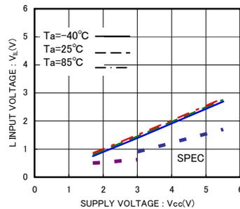
Fig.4 'L' input voltage  $V_{IL}$  (A2,SCL,SDA,WP)
