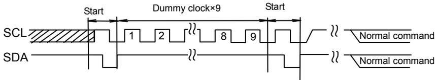
Fig.385-(b) The case of START+9 Dummy clock + START + command input
