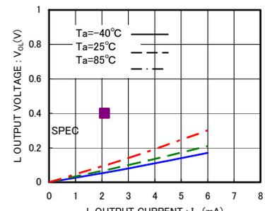
Fig.5 'L' output voltage  $V_{OL}$ - $I_{OL}$  ( $V_{CC}=1.7V$ )
