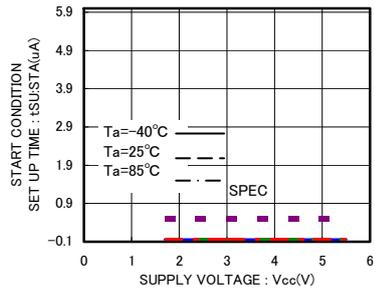
Fig.16 Start Condition Setup Time  $t_{SU:STA}$
