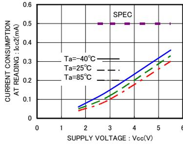
Fig.10 Current consumption at READ operation  $I_{cc2}$  (fsc1=400kHz)
