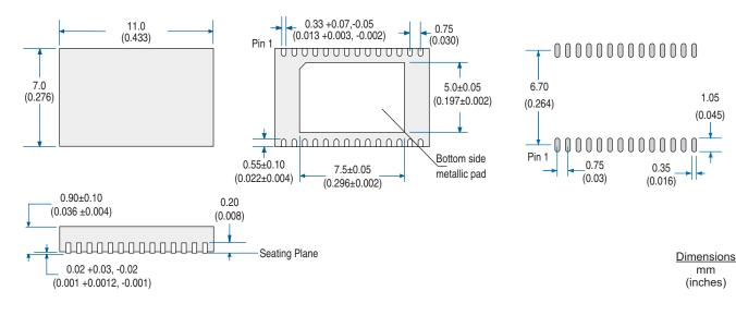
NOTE: As the metallic pad on the bottom of the DFN package is connected to the substrate of the die, Clare recommends that no printed circuit board traces cross this area to avoid potential shorting issues.
