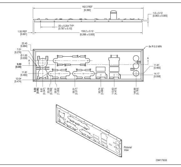
Figure 27. I/O Shield Dimensions for Boards with the 6-Channel (5.1) Audio Subsystem
