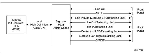
Figure 10 is a block diagram of the 8-channel (7.1) audio subsystem.
