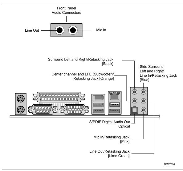
Figure 9. Front/Back Panel Audio Connector Options for 8-Channel (7.1) Audio Subsystem
