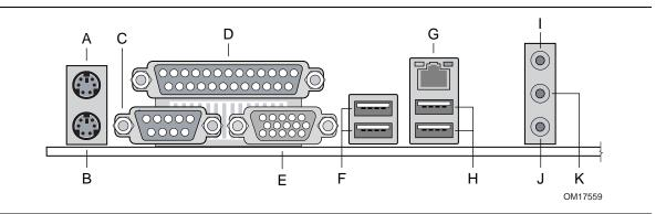
Figure 19. Back Panel Connectors for 6-Channel (5.1) Audio Subsystem
