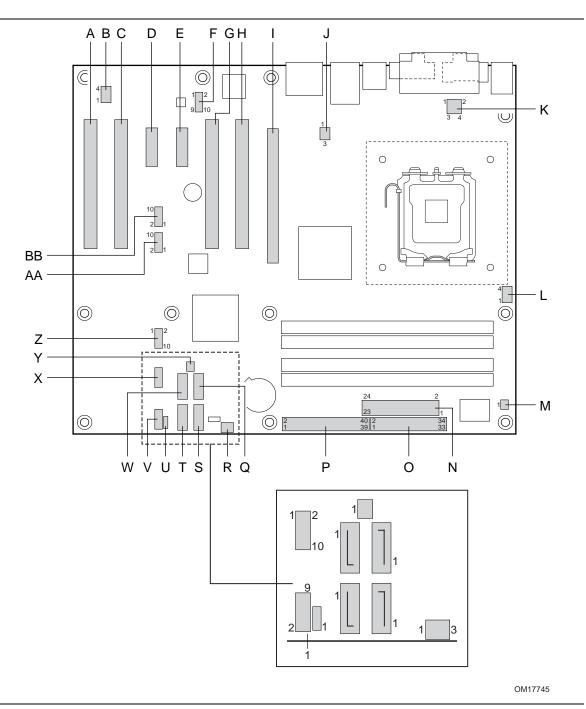
Figure 20. Component-side Connectors
