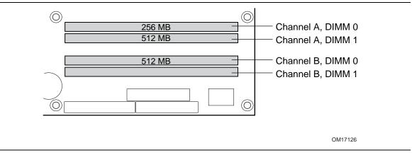
Figure 8. Single Channel (Asymmetric) Mode Configuration with Three DIMMs
