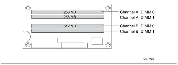
Figure 5. Dual Channel (Interleaved) Mode Configuration with Three DIMMs
