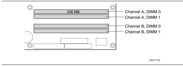
Figure 7. Single Channel (Asymmetric) Mode Configuration with One DIMM
