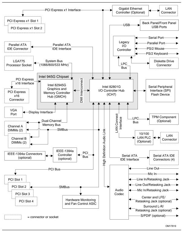
Figure 2. Block Diagram
