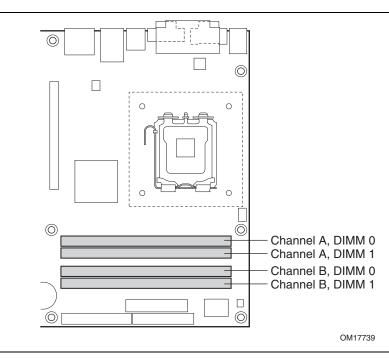
Figure 3. Memory Channel and DIMM Configuration
