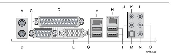
Figure 18. Back Panel Connectors for 8-Channel (7.1) Audio Subsystem
