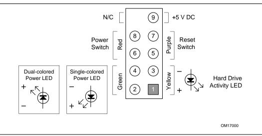
Figure 21. Connection Diagram for Front Panel Connector
