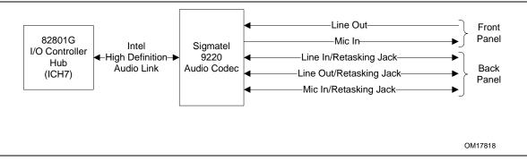
Figure 12. 6-Channel (5.1) Audio Subsystem Block Diagram
