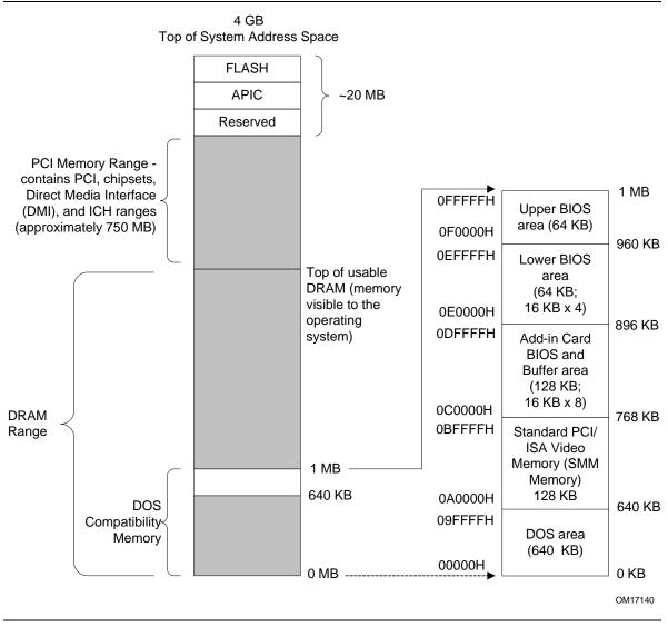
Figure 17. Detailed System Memory Address Map
