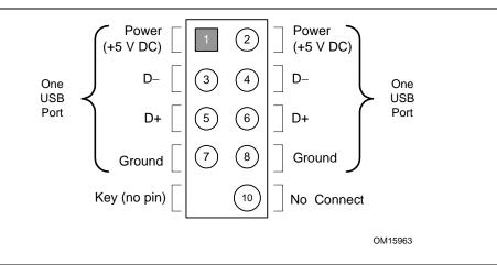
Figure 22. Connection Diagram for Front Panel USB Connectors
