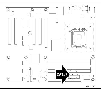
Figure 16. Location of the Standby Power Indicator LED
