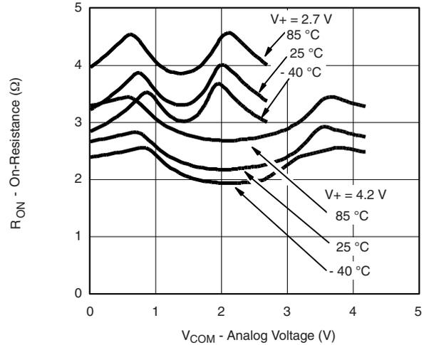
**R<sub>ON</sub> vs. Analog Voltage and Temperature**
