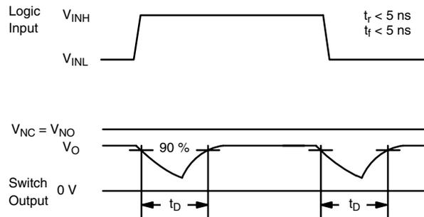
Figure 2. Break-Before-Make Interval
