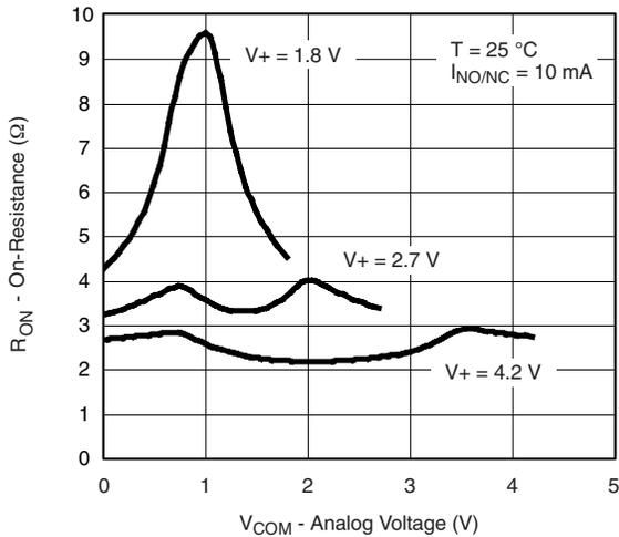
**R<sub>ON</sub> vs. V<sub>COM</sub> and Supply Voltage**
