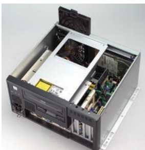
Solid disk drive housing & easy-to-maintain fan filter
