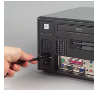
Plug ring-lock securely fastens the power cord
