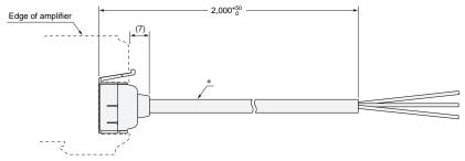
\* Cable 4-dia. vinyl-insulated round cable with 3 conductors (Conductor cross section: 0.2 mm², Insulator diameter: 1.1 mm)
