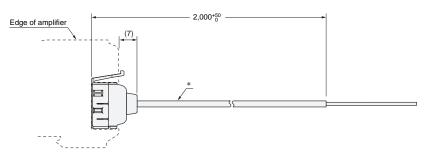
\* Cable 2.6-dia. vinyl-insulated round cable with 1 conductors (Conductor cross section: 0.2 mm², Insulator diameter: 1.1 mm)
