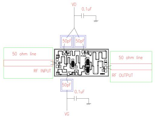
The length of RF wires should be as short as possible. Use at least two wires between RF pad and 50 ohm line and separate the wires to minimize the mutual inductance.
