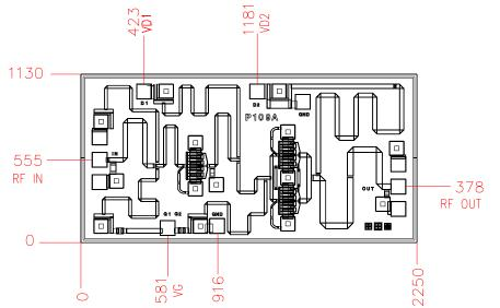
Chip Size 1130 x 2250 microns Chip Thickness:  $85 \pm 15$  microns PAD Dimensions: 100 x 100 microns All Dimensions in Microns
