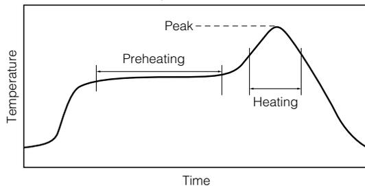
For soldering (Example : Sn-37Pb)
