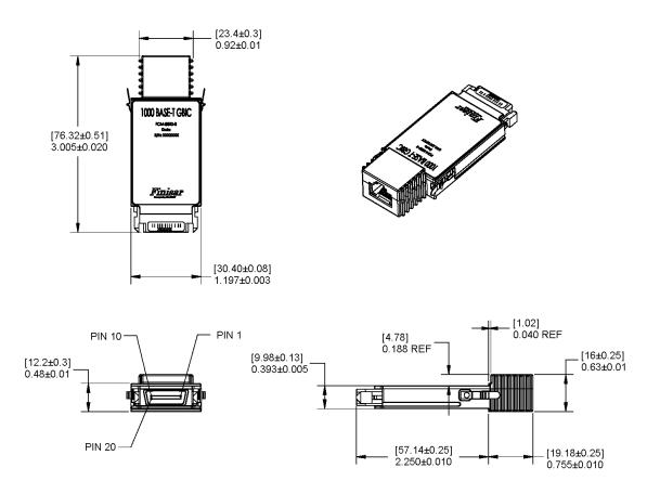
Figure 1. FCM-8520/8521-3 mechanical dimensions
