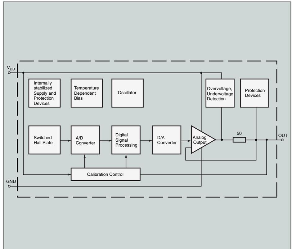
Fig. 1: Block diagram of the HAL 1821/1822/1823
