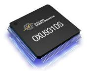
The OXU931DS is a single chip solution for bridging between USB 2.0 or eSATA and hard disks.
