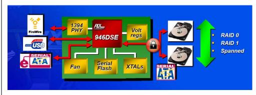
The integrated hardware RAID engine supports a range of RAID modes which deliver maximum performance (RAID 0), maximum data protection (RAID 1) or maximum capacity (spanning).
