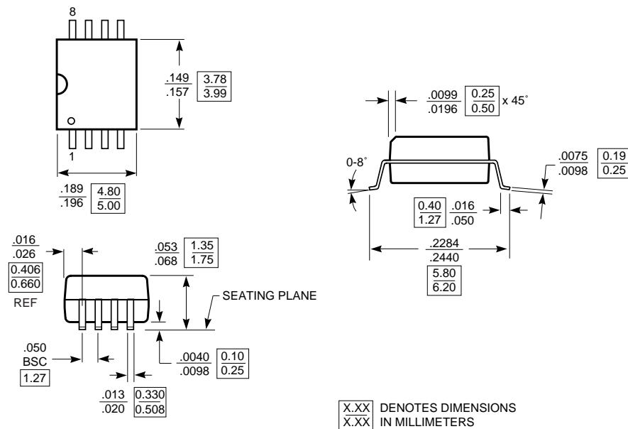
**Packaging Mechanical: 8-Pin MSOP (U)**
