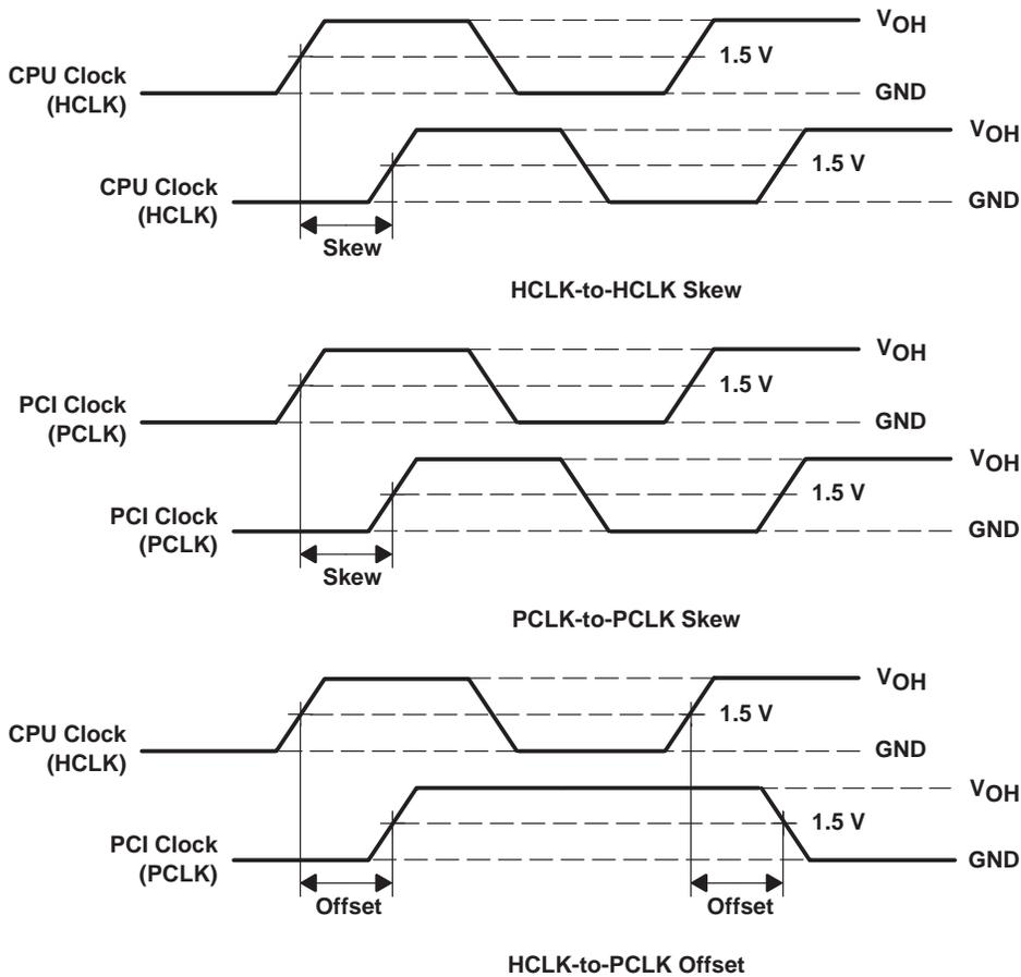
**Figure 2. Waveforms for Calculation of  $t_{skew}$  and  $t_{offset}$**
