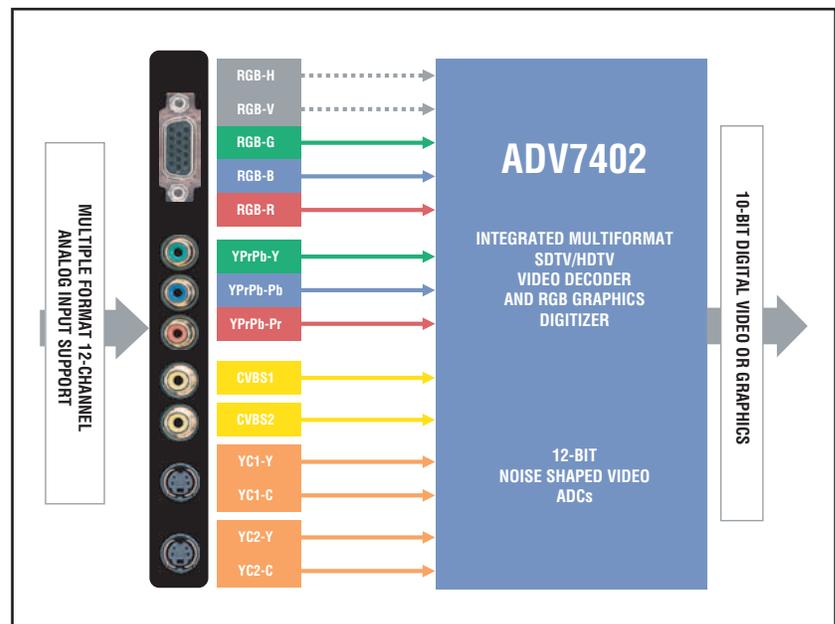
Evaluation kits for the ADV7402 and ADV7400 are now available from Analog Devices. All kits include the equipment necessary to start prototyping with those devices. With the on-board ADuC831 microcontroller, each kit comes ready programmed for standalone operation, including pre-programmed auto detection and mode selection via the on-board rotary hex switches.
