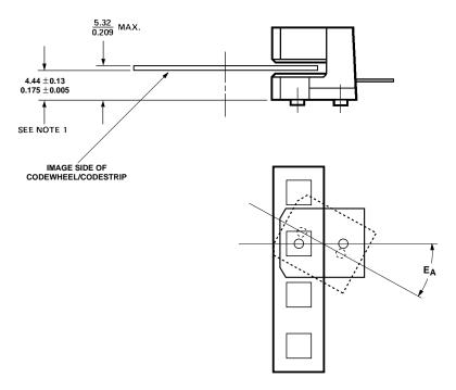
For linear motion, angular misalignment,  $\mathbf{E}_{\mathbf{A}}$ , must be  $\leq \pm \ 2$  degrees to achieve Encoding Characteristics.
