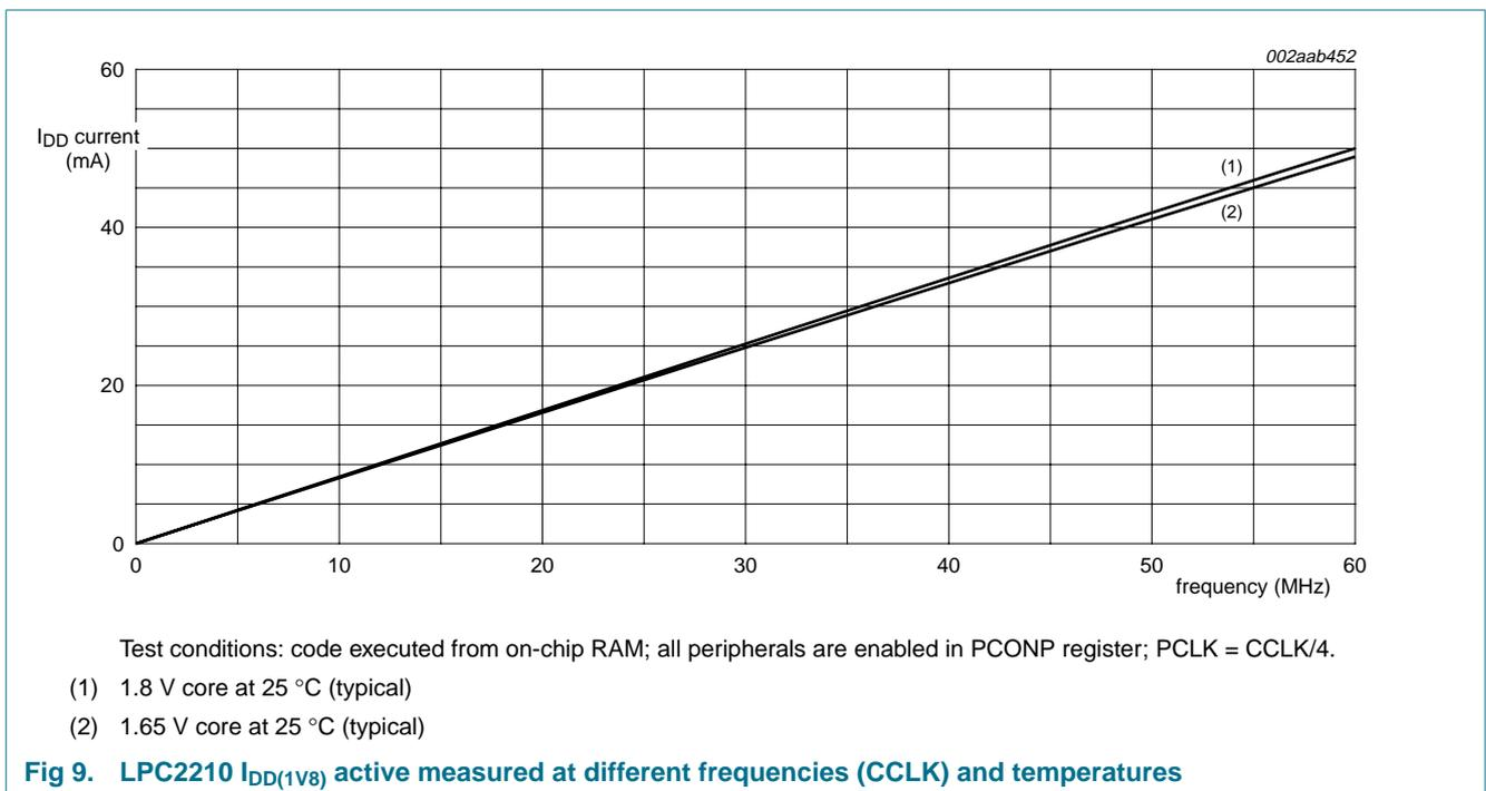
Fig 9. LPC2210  $I_{DD(1V8)}$  active measured at different frequencies (CCLK) and temperatures
