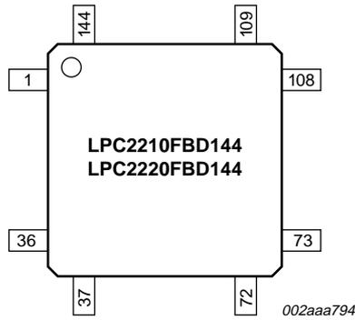
Fig 2. Pin configuration for LQFP144
