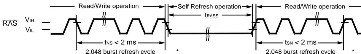
\* read/write operation can be performed non refresh time within  $t_{NS}$  or  $t_{SN}$
