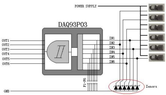
Above picture shows external proximity switch sensors connect to the DAQ93P03 whereby the sensors are commonly power supplied with 8volts regulated PSU and return signals are directly feed into each input channel of the chip. For mechanical switches, the power supply is recommended to 5Volts.
