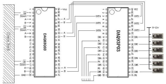
Above figure shows a typical connection for a counter board, DAQ83Q03 and DAQ93P03 whereby filters is to be connected as per requirement of specific project.
