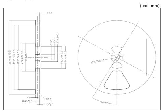
\*1: Material: PS, Conductivity:  $10^4 \Omega \sim 10^5 \Omega$
