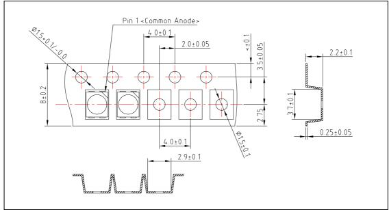
\*1: Material: PS, Conductivity:  $10^9 \Omega \sim 10^{12} \Omega$
