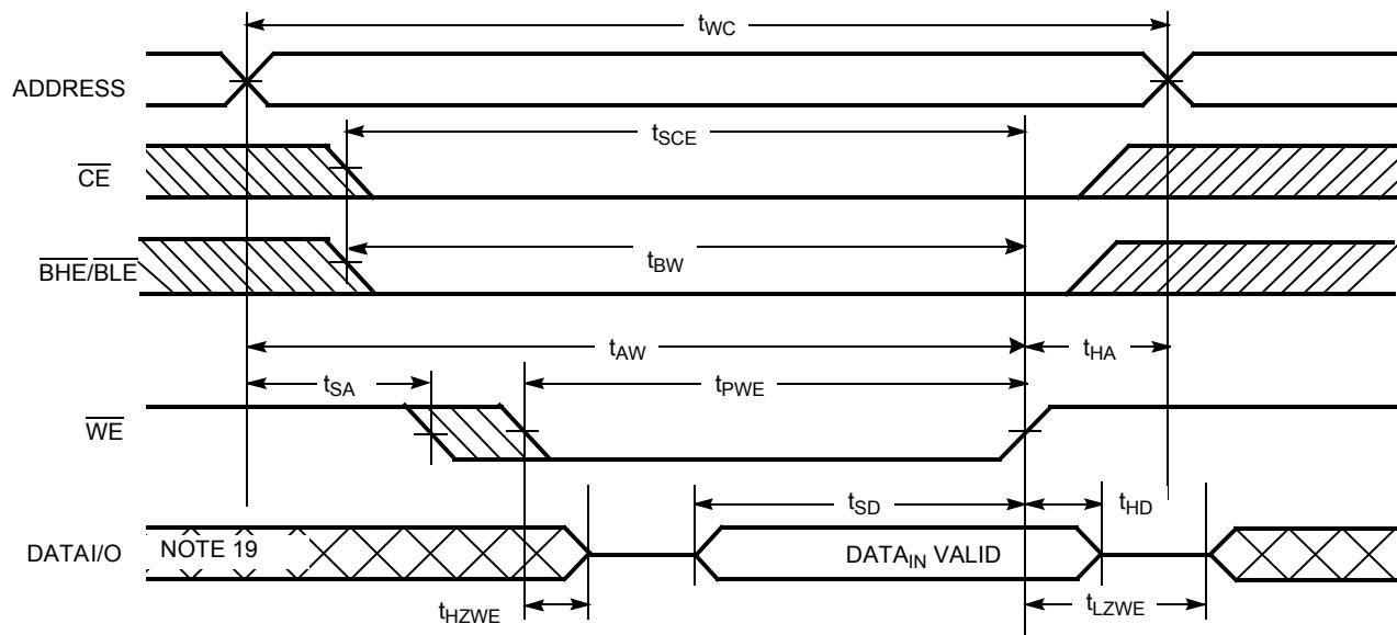
**Write Cycle No. 4 (BHE-/BLE-controlled,  $\overline{\text{OE}}$  LOW)<sup>[17, 18]</sup>**
