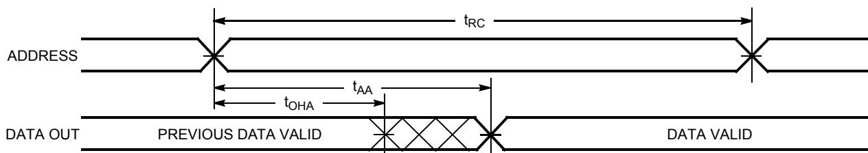
**Read Cycle No. 2 ( $\overline{OE}$  Controlled)<sup>[15, 16]</sup>**
