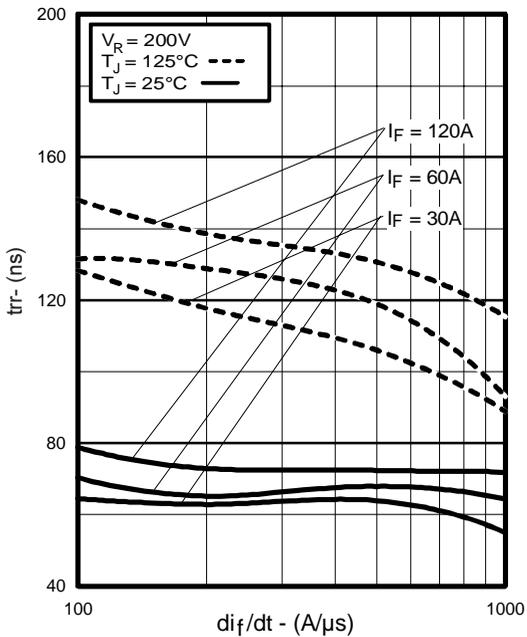
**Fig. 5** - Typical Reverse Recovery vs.  $di_f/dt$ , (per Leg)
