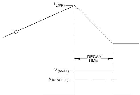
**Fig. 11 - Avalanche Test Circuit and Waveforms**
