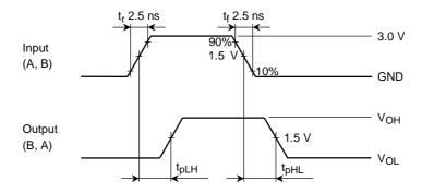
Figure 2 t<sub>pLH</sub>, t<sub>pHL</sub>
