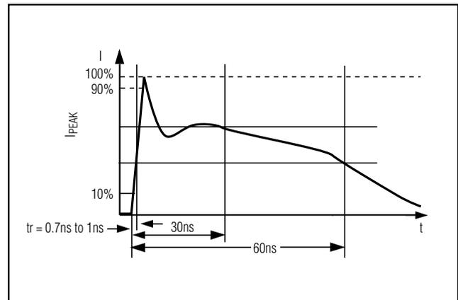
Figure 9. IEC 1000-4-2 ESD Generator Current Waveform
