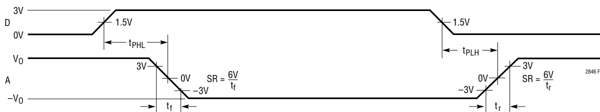
Figure 15. V.28 Driver Propagation Delays
