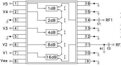
DC Blocking Capacitors C1 & C2 are required on RF1 & RF2. Choose C1 = C2 =  $100 \text{ pF} \sim 0.1 \text{ uF}$  to allow lowest customer specific frequency to pass with minimal loss. R1= 5K Ohm is required to supply voltage to the circuit through either Pin 11 or Pin 14.
