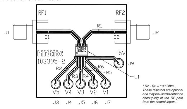
The circuit board used in the final application should use RF circuit design techniques. Signal lines should have 50 ohm impedance while the package ground leads and exposed paddle should be connected directly to the ground plane similar to that shown. A sufficient number of via holes should be used to connect the top and bottom ground planes. The evaluation circuit board shown is available from Hittite upon request.
