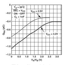
TPC 12. Charge Injection vs. Source Voltage
