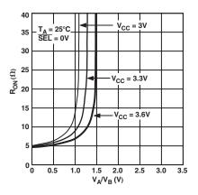
TPC 3. On Resistance vs. Input Voltage
