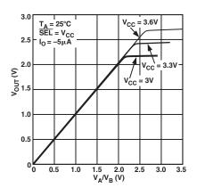
TPC 6. Pass Voltage vs.  $V_{CC}$
