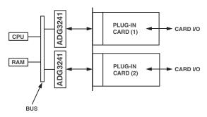
Figure 12. ADG3241 in a Hot Plug Application
