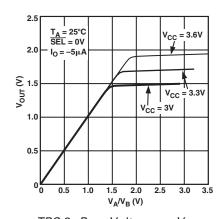
TPC 8. Pass Voltage vs.  $V_{CC}$
