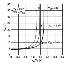
TPC 1. On Resistance vs. Input Voltage
