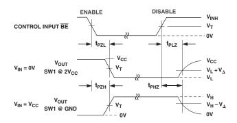
Figure 3. Enable and Disable Times
