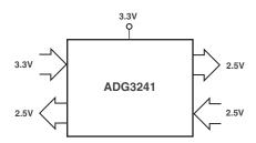
Figure 5. 3.3 V to 2.5 V Voltage Translation,  $\overline{SEL} = V_{CC}$  In this case, the output will be limited to 2.5 V, as shown in Figure 6. This device can be used for translation from 2.5 V to 3.3 V devices and also between two 3.3 V devices.
