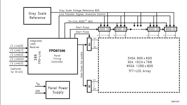
FIGURE 1. Block Diagram of the LCD Module
