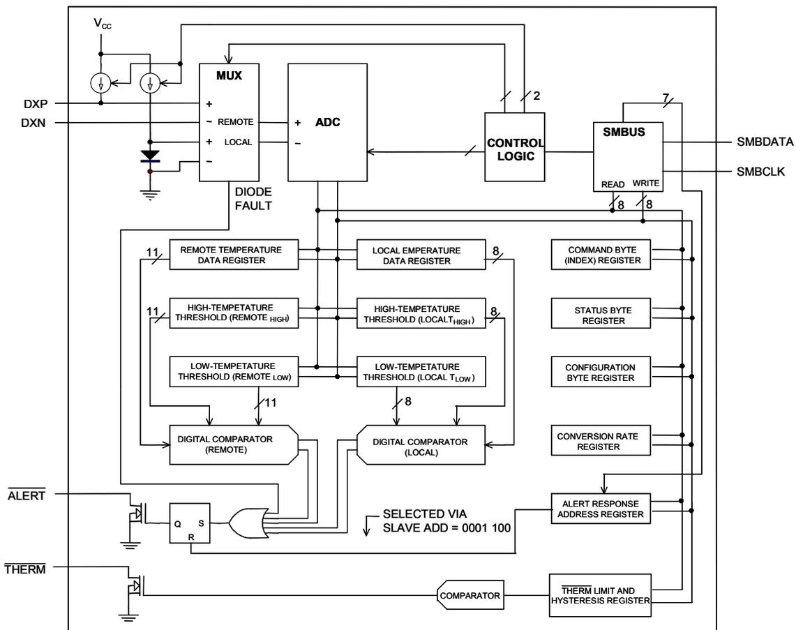
**Figure 1. Functional Diagram**
