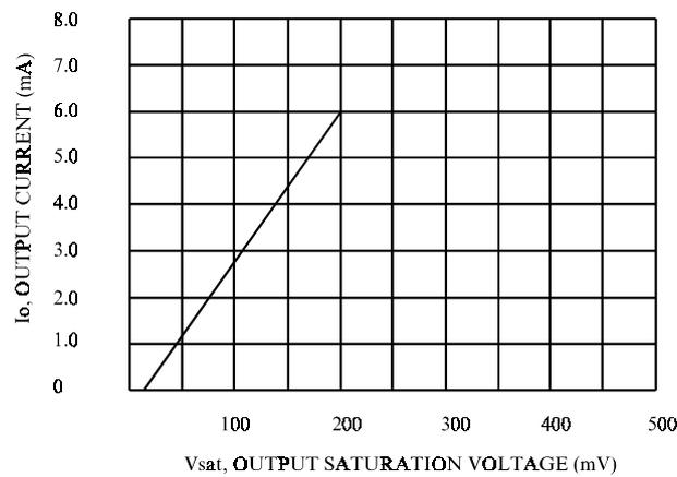
**Figure 3. Output Sink Current versus Output Saturation Voltage**
