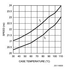
FIGURE 9. Speed vs Case Temperature
