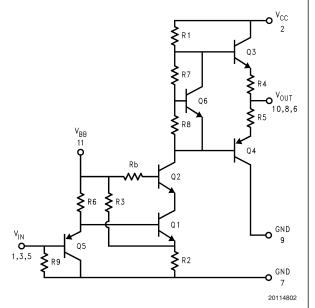
FIGURE 2. Simplified Schematic Diagram (One Channel)
