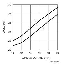
FIGURE 7. Speed vs Load Capacitance
