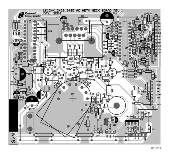
FIGURE 15. LM2423/LM1246/LM2485 DTV Demonstration Board Layout
