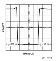
FIGURE 12. LM2423 Cathode Response
