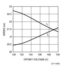
FIGURE 8. Speed vs Offset
