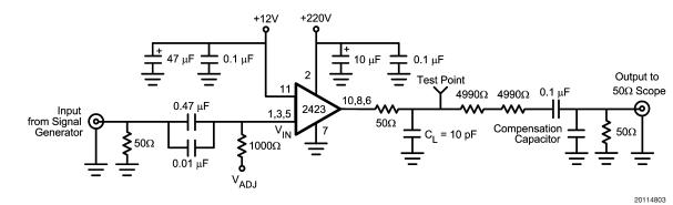
Note: 10 pF load includes parasitic capacitance.
