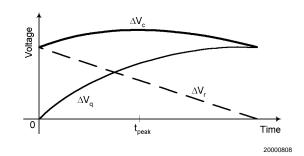
FIGURE 4. Delta Output Voltage Components
