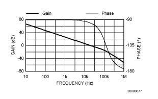
FIGURE 13. Example Loop Transfer Function
