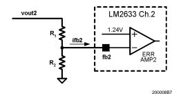
FIGURE 17. Setting the Ch2 Output Voltage
