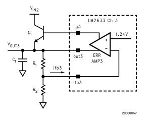
FIGURE 19. Channel 3 Controlling an LDO
