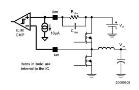
FIGURE 1. Current Limit Method
