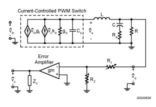
FIGURE 7. Small Signal Model of Buck Regulators
