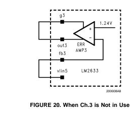
The error amplifier of Channel 3 has a DC gain of 83 dB, and a unity-gain bandwidth of 200 kHz. See the plots in *Figure 21*.
