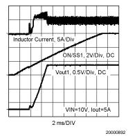
Load Transient Response (Ch 1, Typical Application, VOUT1 = 1.6V)
