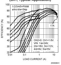
Efficiency vs Load Current (Ch2, Typical Application, FPWM = 1)
