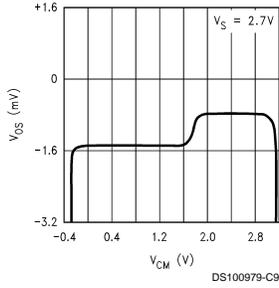
**Offset Voltage vs. Common Mode Voltage**
