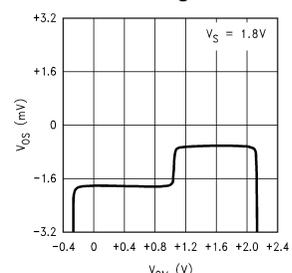
**Typical Performance Characteristics** Unless otherwise specified,  $V_S = +5V$ , single supply,  $T_A = 25^\circ C$ . (Continued)
