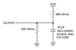
Figure 1: AC Output Loading
