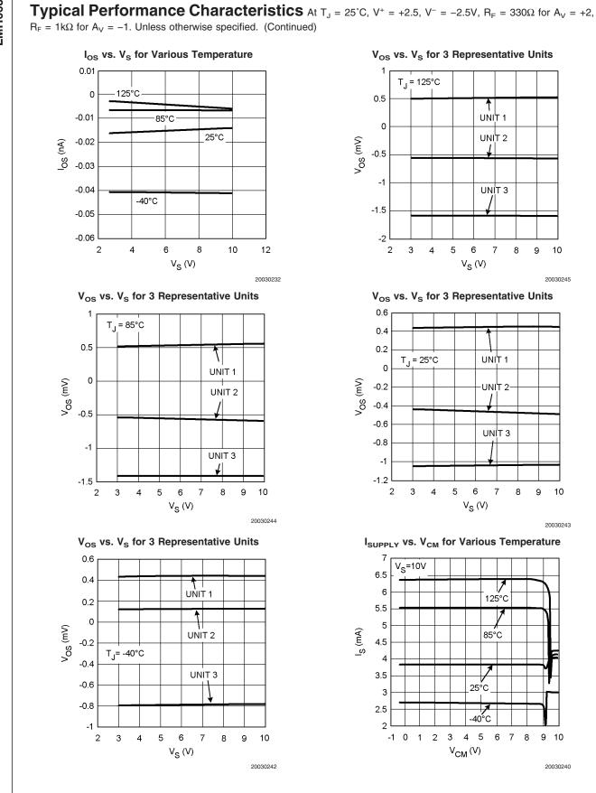
**Typical Performance Characteristics** At  $T_J = 25^{\circ}C$ ,  $V^+ = +2.5$ ,  $V^- = -2.5V$ ,  $R_F = 330\Omega$  for  $A_V = +2$ ,  $R_F = 1k\Omega$  for  $A_V = -1$ . Unless otherwise specified. (Continued)
