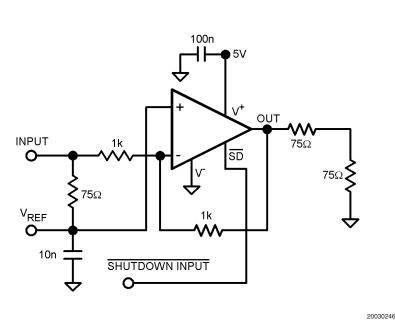
FIGURE 1. Typical Single Supply Schematic
