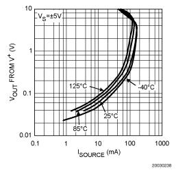
Output Sourcing Saturation Voltage vs.  $I_{OUT}$ for Various Temperature
