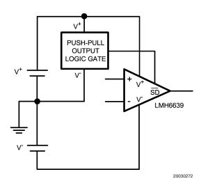
FIGURE 5. Shutdown Interface (Dual Supplies)
