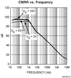
**Typical Performance Characteristics** At  $T_J = 25^{\circ}C$ ,  $V^+ = +2.5$ ,  $V^- = -2.5V$ ,  $R_F = 330\Omega$  for  $A_V = +2$ ,  $R_F = 1k\Omega$  for  $A_V = -1$ . Unless otherwise specified. (Continued)
