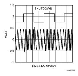
FIGURE 3. Switching between 5 and 10MHz
