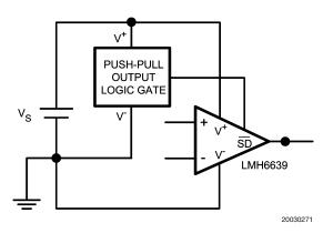
FIGURE 4. Shutdown Interface (Single Supply)
