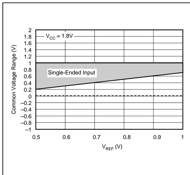
FIGURE 2. Single-Ended Input—Common Voltage Range vs V<sub>REF</sub>.
