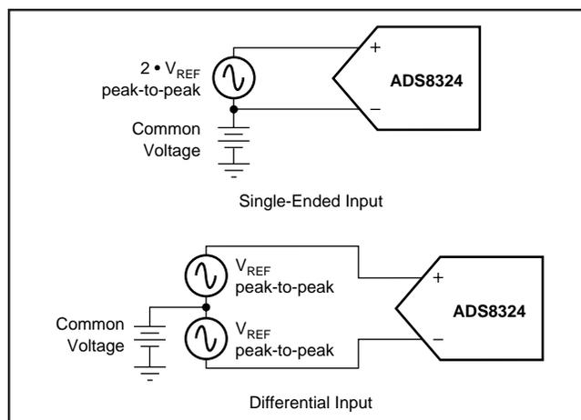
FIGURE 1. Methods of Driving the ADS8324—Single-Ended or Differential.
