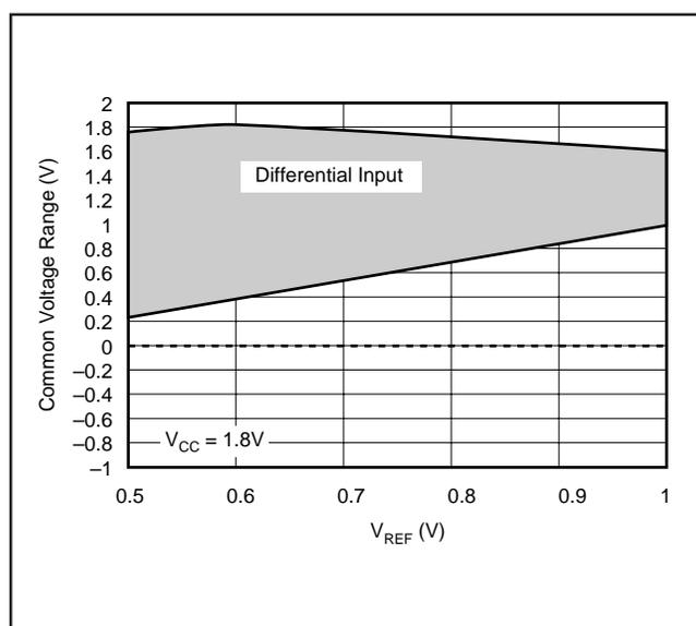
FIGURE 3. Differential Input—Common Voltage Range vs V<sub>REF</sub>.
