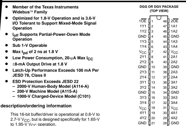
The device can be used as four 4-bit buffers, two 8-bit buffers, or one 16-bit buffer. It provides inverting outputs and symmetrical active-low output-enable ( $\overline{OE}$ ) inputs.
