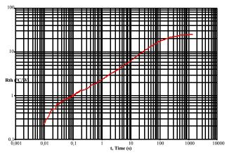
Figure 20. 33887 Thermal Response, HSOP Package
