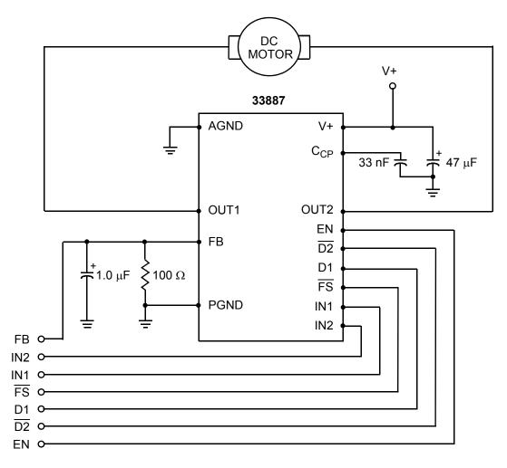
Figure 21. 33887 Typical Application Schematic
