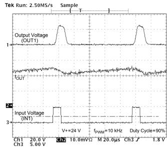
Figure 16. Output Voltage and Current vs. Input Voltage at V+ = 24 V, PMW Frequency of 10 kHz, and Duty Cycle of 90%
