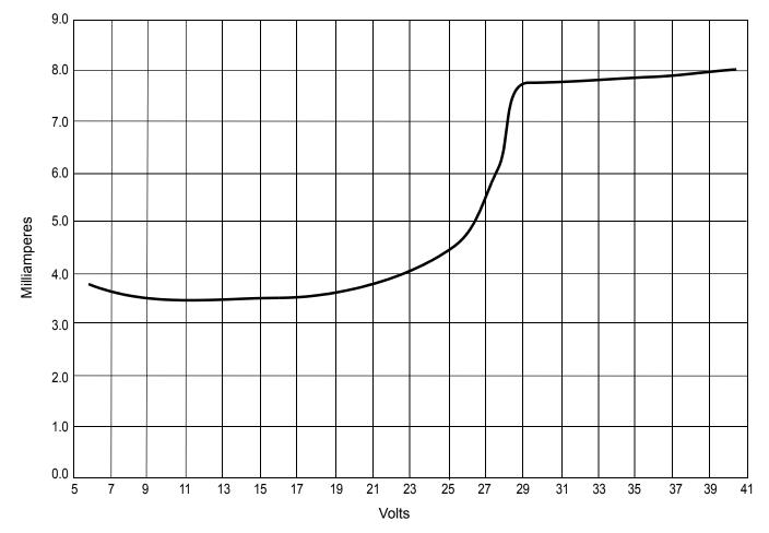
Figure 10. Typical Quiescent Supply Current Versus V+
