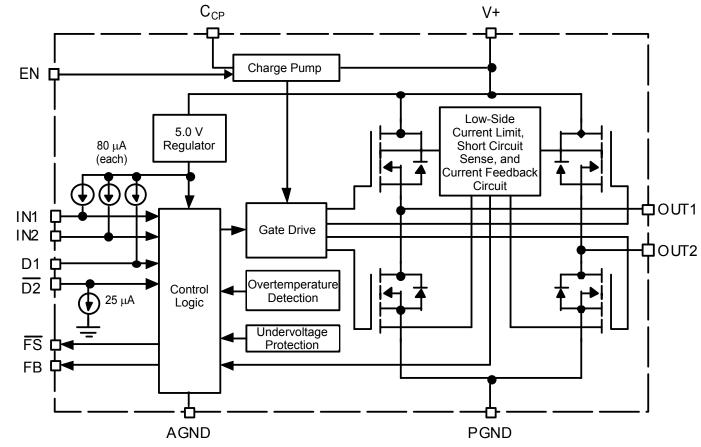
Figure 1. 33887 Simplified Internal Block Diagram
