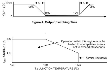
Figure 5. Active Current Limiting Versus Temperature (Typical)
