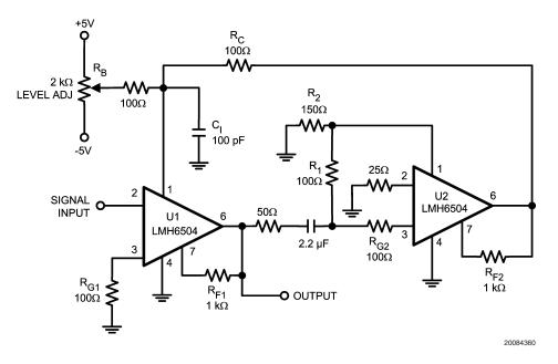
FIGURE 9. Automatic Gain Control Circuit #2
