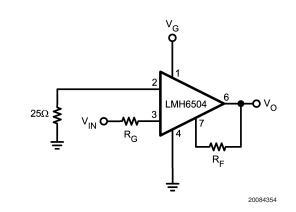
FIGURE 4. Inverting Amplifier
