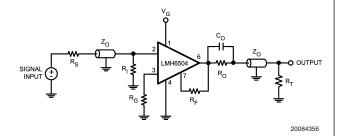
FIGURE 5. TRANSMISSION LINE MATCHING
