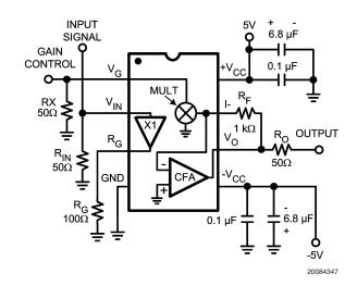
FIGURE 1. LMH6504 Typical Application and Block Diagram
