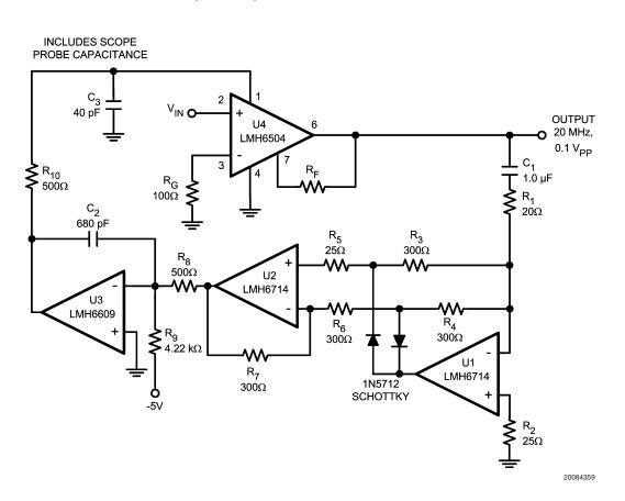
FIGURE 8. Automatic Gain Control Circuit #1
