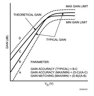
FIGURE 2. LMH6504 Gain Accuracy & Gain Matching Defined
