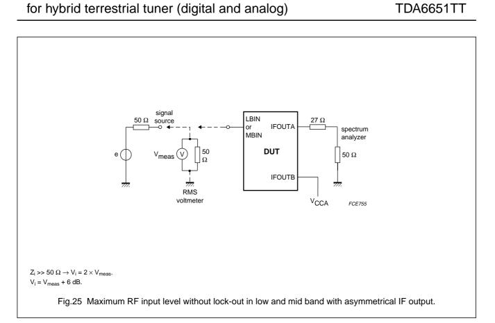
5 V mixer/oscillator and low noise PLL synthesizer
